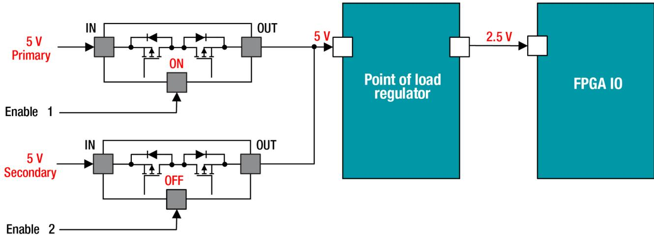
**Figure 1. Block Diagram of a Cold Spring Application**
