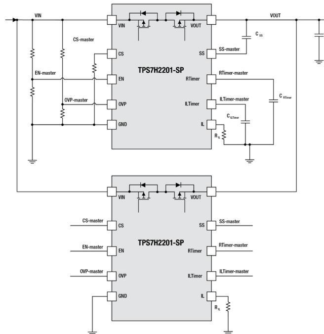
**Figure 2. Block Diagram of a Smart Load Switch Used in Parallel**
