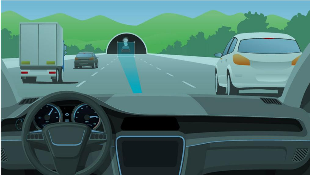
**Figure 2. The Front Radar of the Approaching Car Needs a High-enough Angle Resolution to Differentiate between the Tunnel and the Stopped Vehicle. mmWave Sensors Can See through Any Visibility Conditions, like Smoke.**
