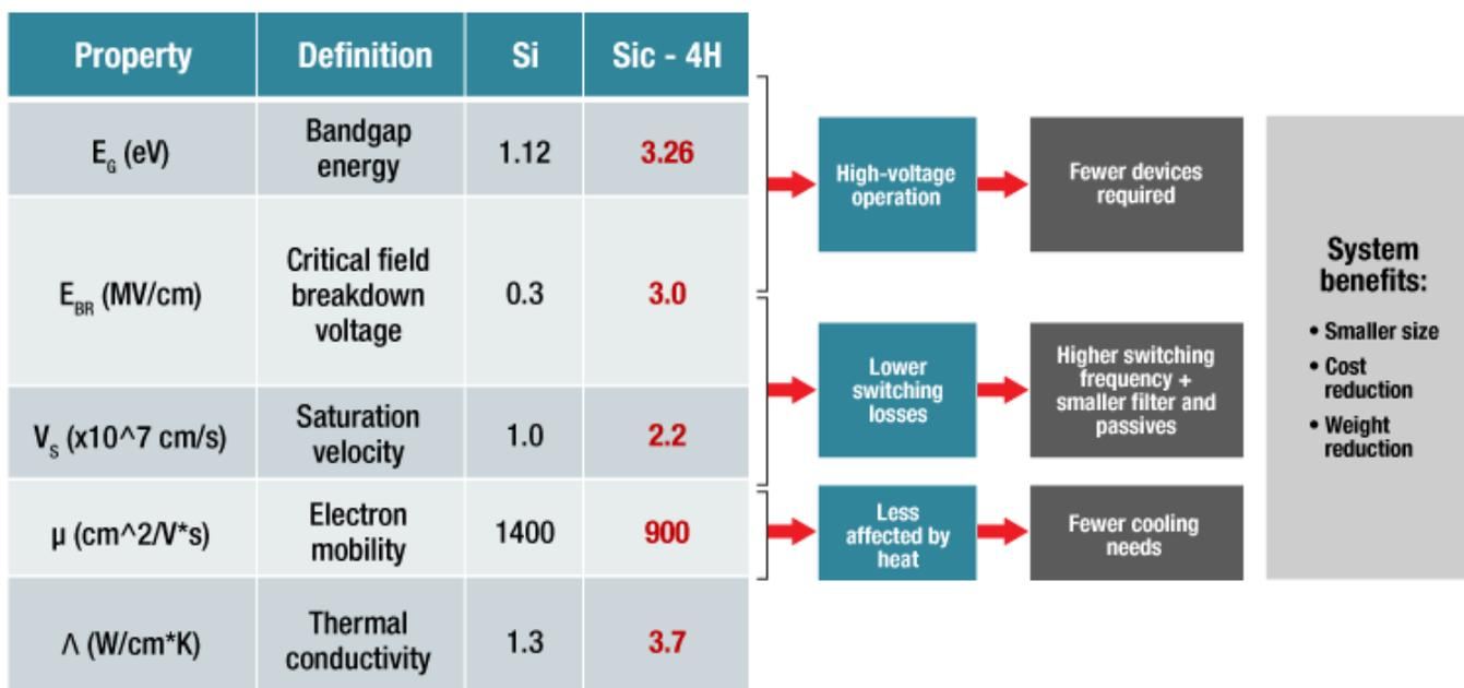
**Figure 2. The Benefits of SiC for Increasing Power Density in Charging Stations**
