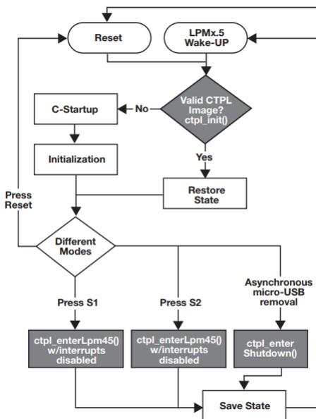
**Figure 2. Flow of an algorithm using the CTPL library**
