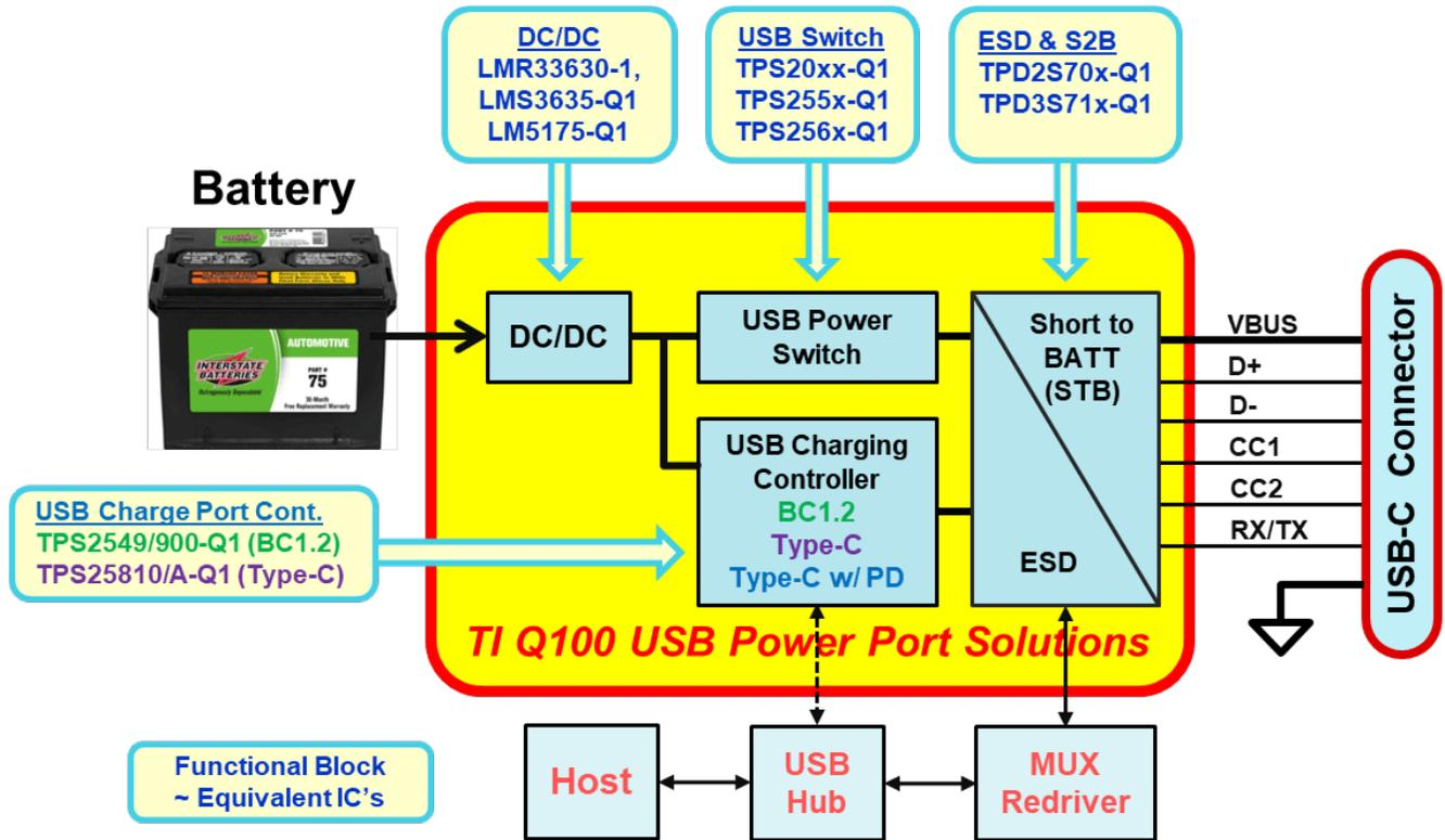
**Figure 2. Equivalent functions of TPS25830-Q1 and TPS25831-Q1 devices**
