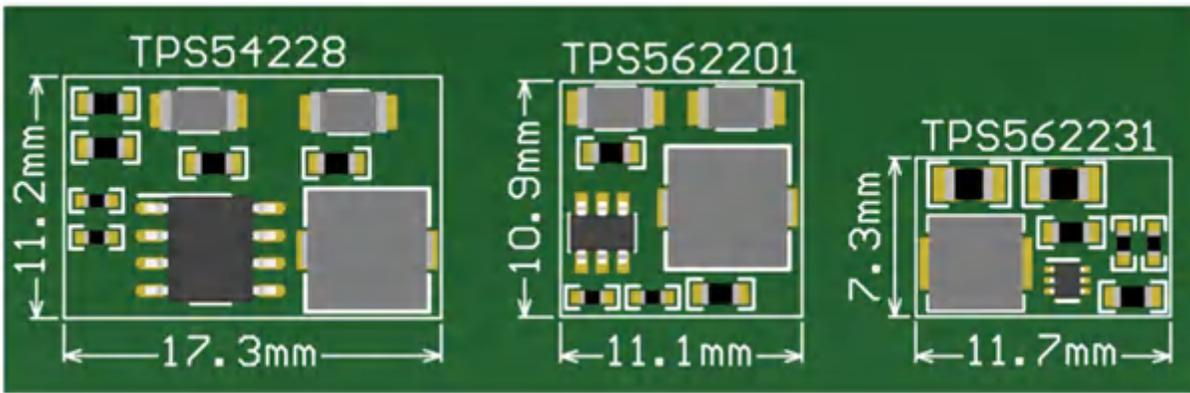
**Figure 3. Solution sizes of converters with different packages**
