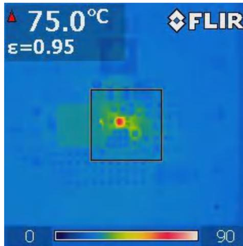
**Figure 4. Thermal image of the TPS562231 with a 12-V input voltage**
