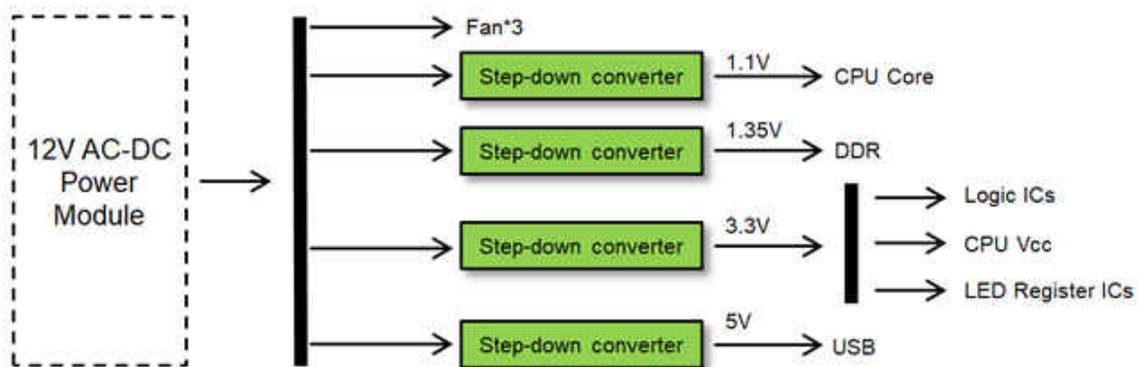
**Figure 2. Power-stage architecture of an embedded system**
