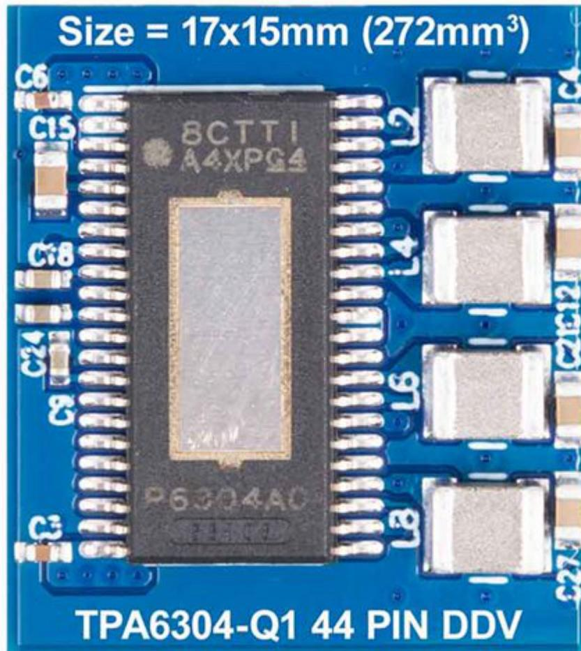
**Figure 2. The TPA6304-Q1 Four-channel Class-D Amplifier**
