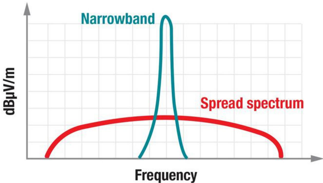
**Figure 6. Spread-spectrum Technology Background**
