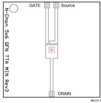
Max  $R_{\theta JA} = 125^{\circ}\text{C/W}$
