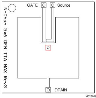
Max  $R_{\theta JA} = 50^{\circ}\text{C/W}$
