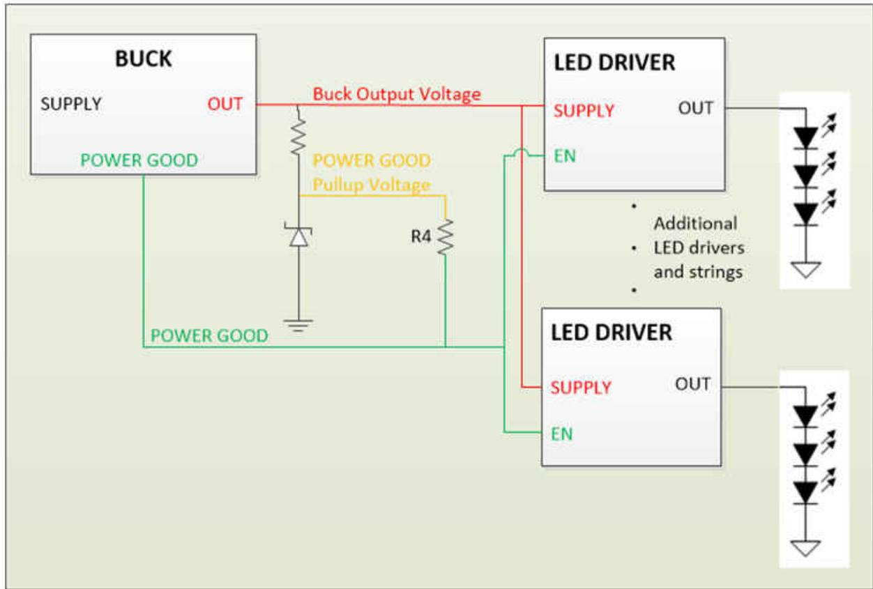
**Figure 4. Connecting POWER GOOD and EN**
