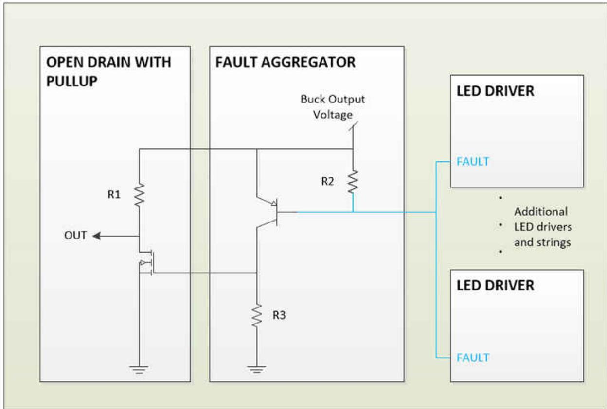
**Figure 3. Fault Aggregator**
