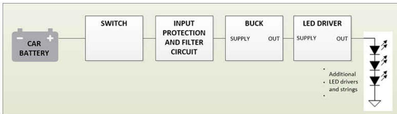
Figure 1. Turn indicator module
