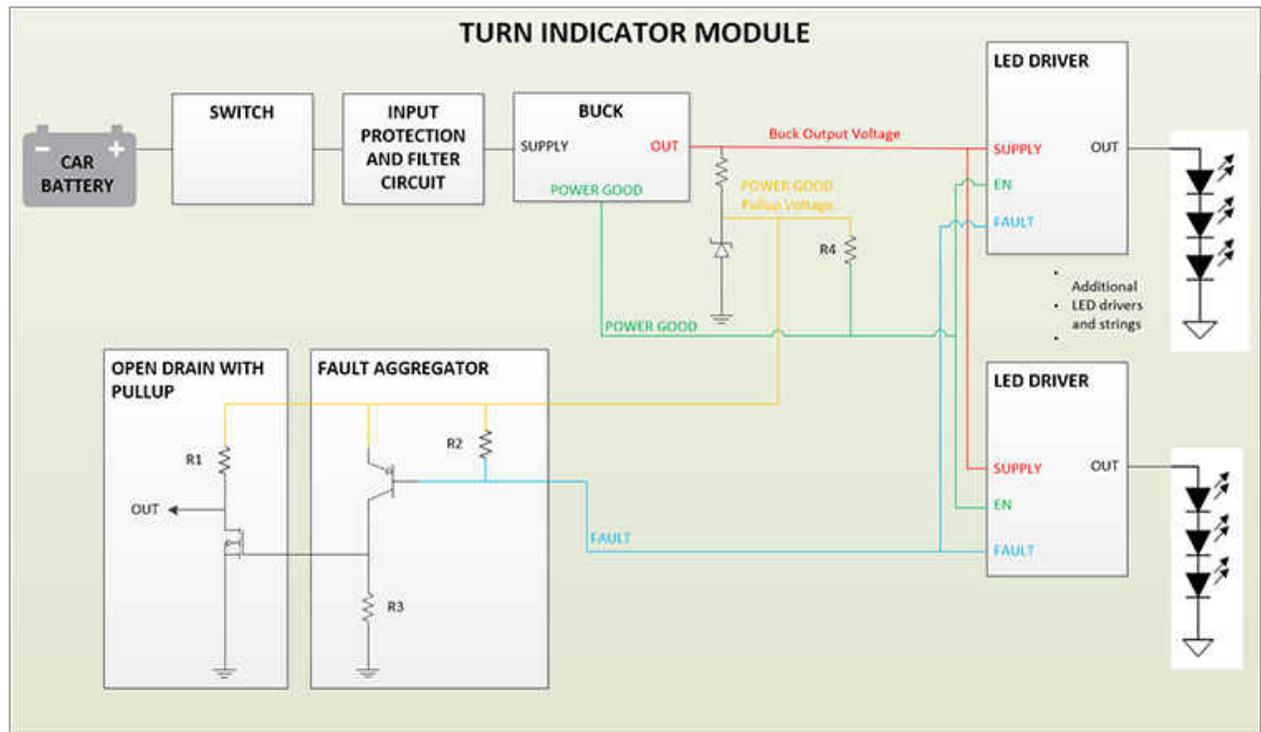
**Figure 5. Disabling OFAF with a Zener Diode and Fault Aggregator**
