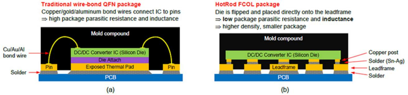
Figure 5. Wire-bond Quad Flat No-lead and FCOL Packages
