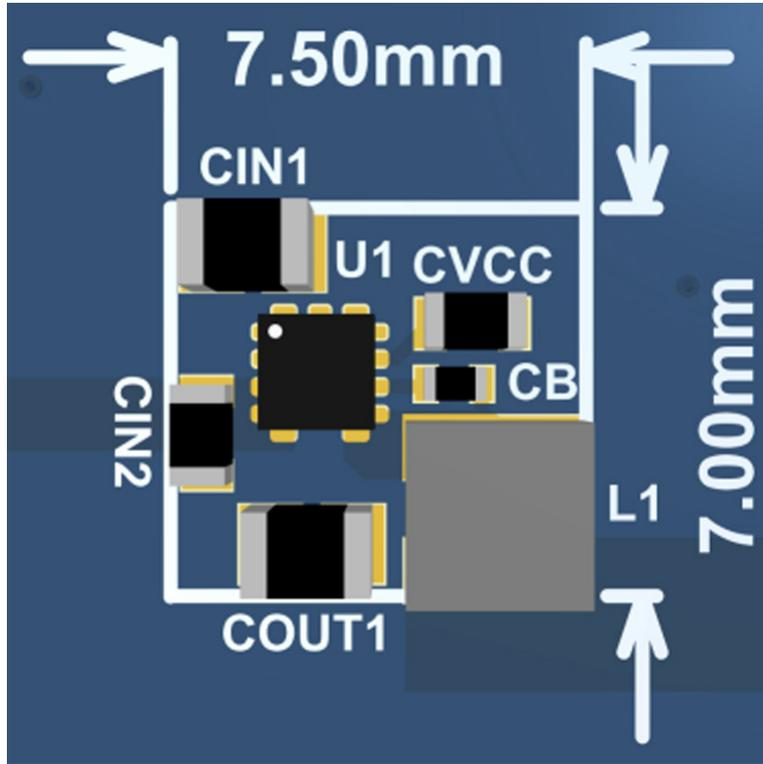
Figure 3. LMR36506 Example Solution Size
