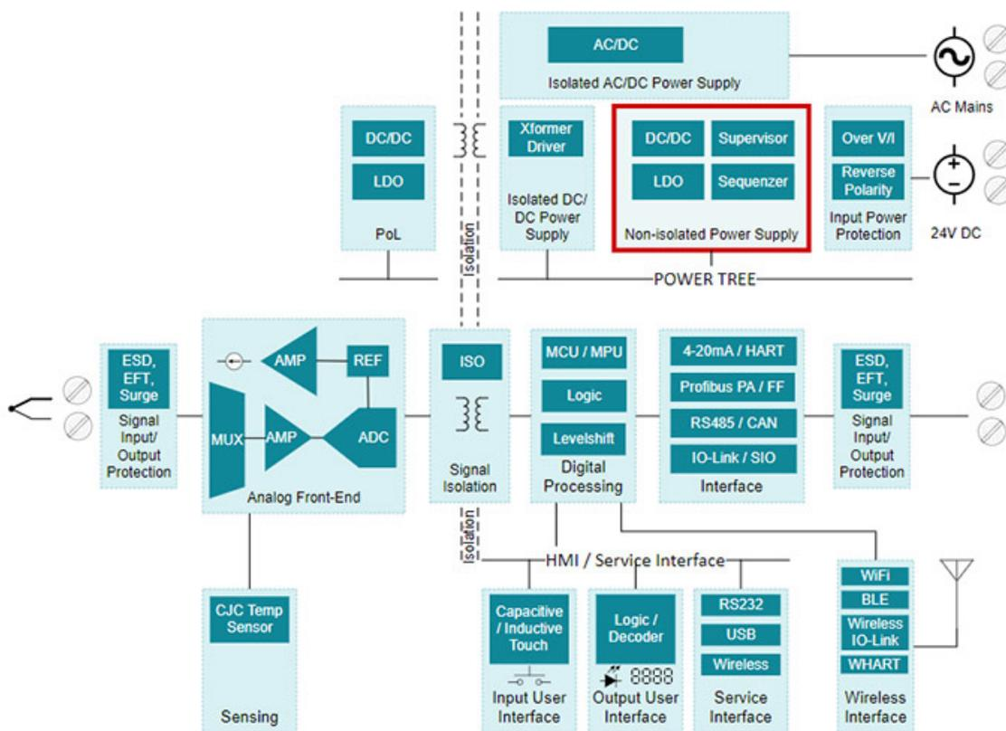
Figure 1. Temperature Transmitter Subsystem
