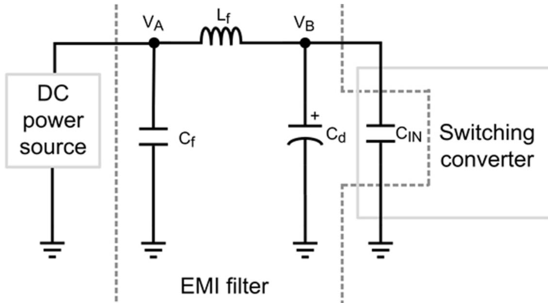
Figure 4. An EMI Filter Structure for DC/DC Converters
