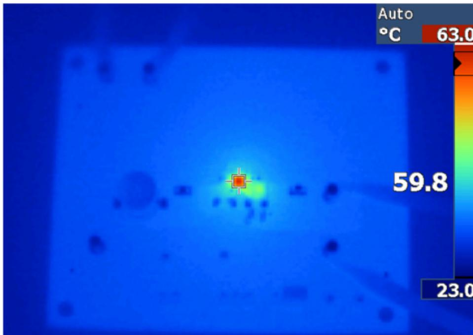
Figure 2. Efficiency and Thermal Performance at 24  $v_{IN}$ , 5  $V_{OUT}$ , 2.1 Mhz at 0.6A
