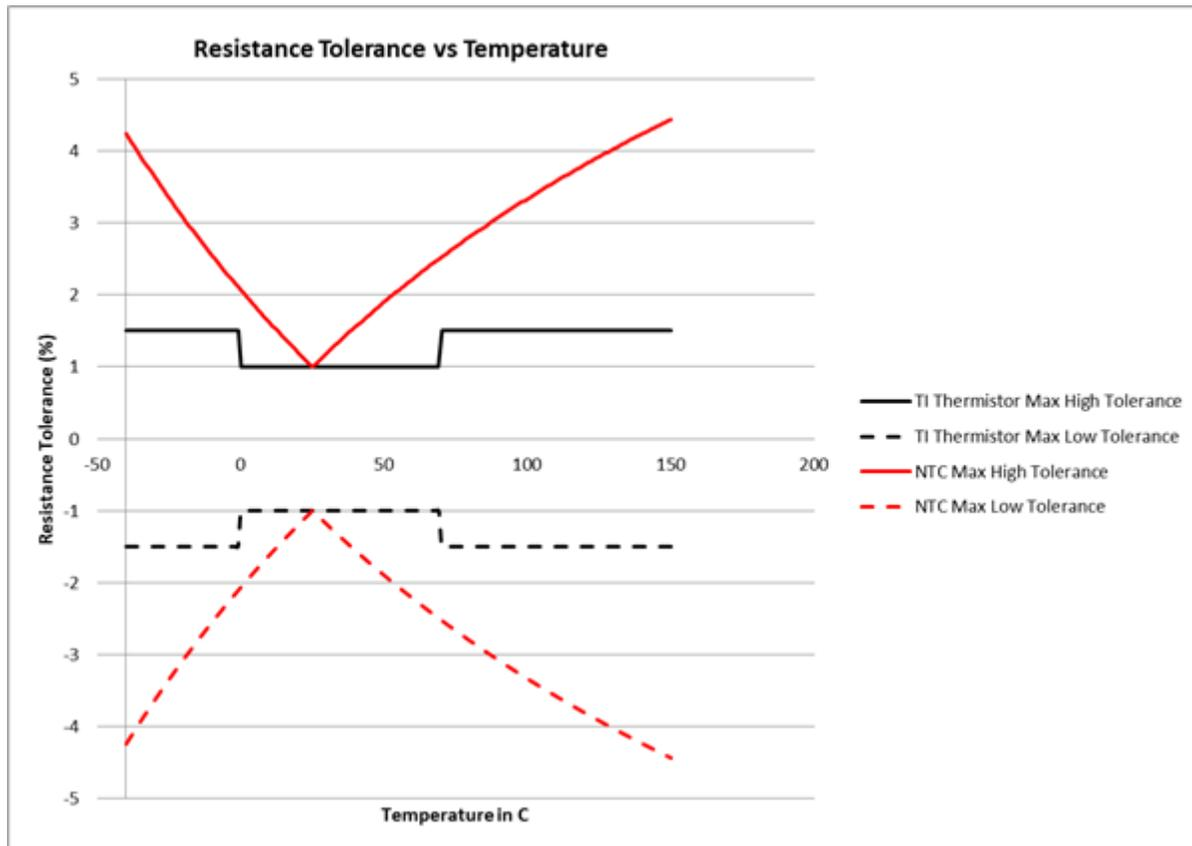
**Figure 1. Resistance Tolerance: NTC vs. the TMP61**
