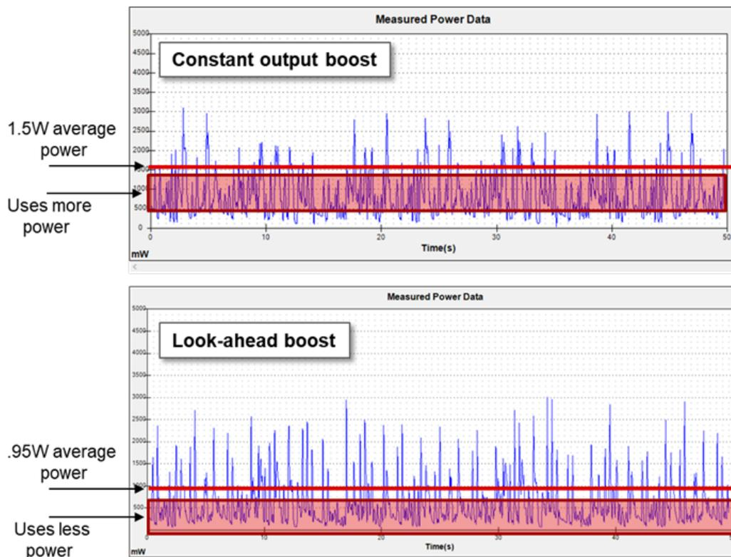
**Figure 2. TI's look-ahead Class-H boost uses half a Watt less power on average**
