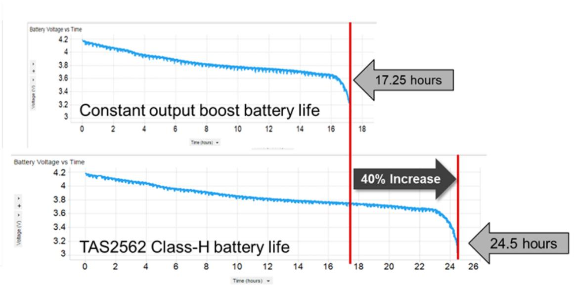
**Figure 1. TI's look-ahead Class-H boost reduces power consumption 40%**
