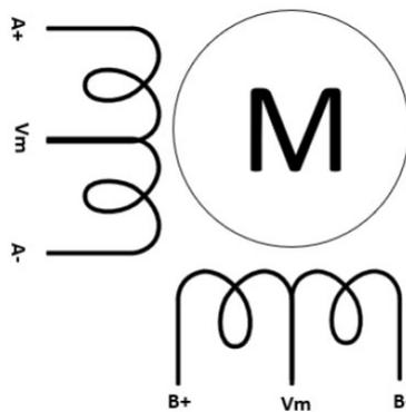
**Figure 1. Six-wire unipolar stepper motor winding connections**
