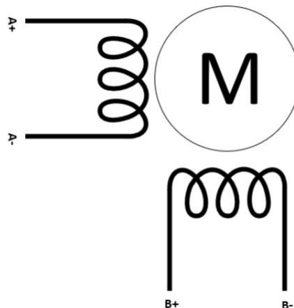
**Figure 3. Four-wire bipolar stepper motor winding connections**
