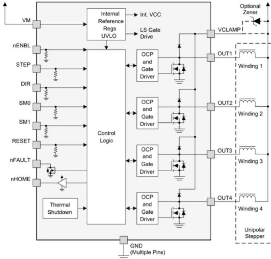
**Figure 2. The DRV8805 wiring when connected to a unipolar motor**
