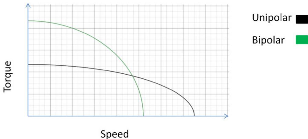
**Figure 5. A unipolar vs. bipolar series stepper motor torque/speed curve**
