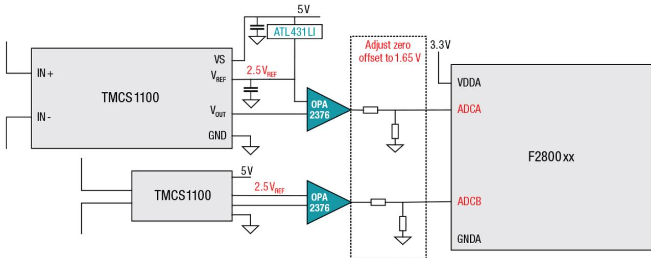
**Figure 1. A common application of Hall-effect current sensors: 3.3 V powering the Hall-effect current sensor (a); 5 V powering the Hall-effect current sensor (b)**
