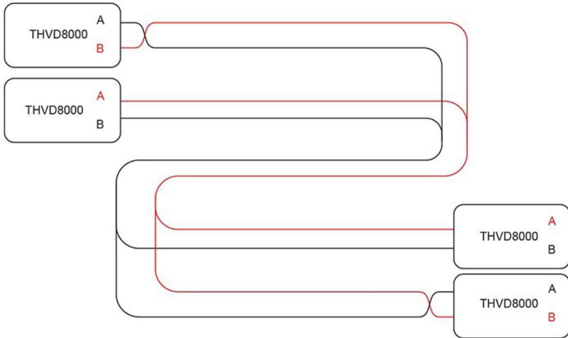
**Figure 3. Polarity-free Mode with the THVD8000**
