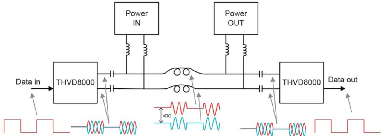
**Figure 1. RS-485 over Power-line Communication Using the THVD8000**
