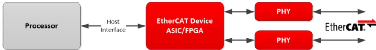
**Figure 2. EtherCAT device with an ASIC/FPGA and external processor**
