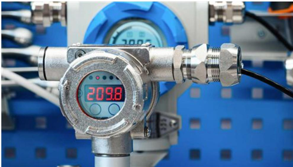
**Figure 1. A Field Sensor That Can Use 10BASE-T1L Ethernet**
