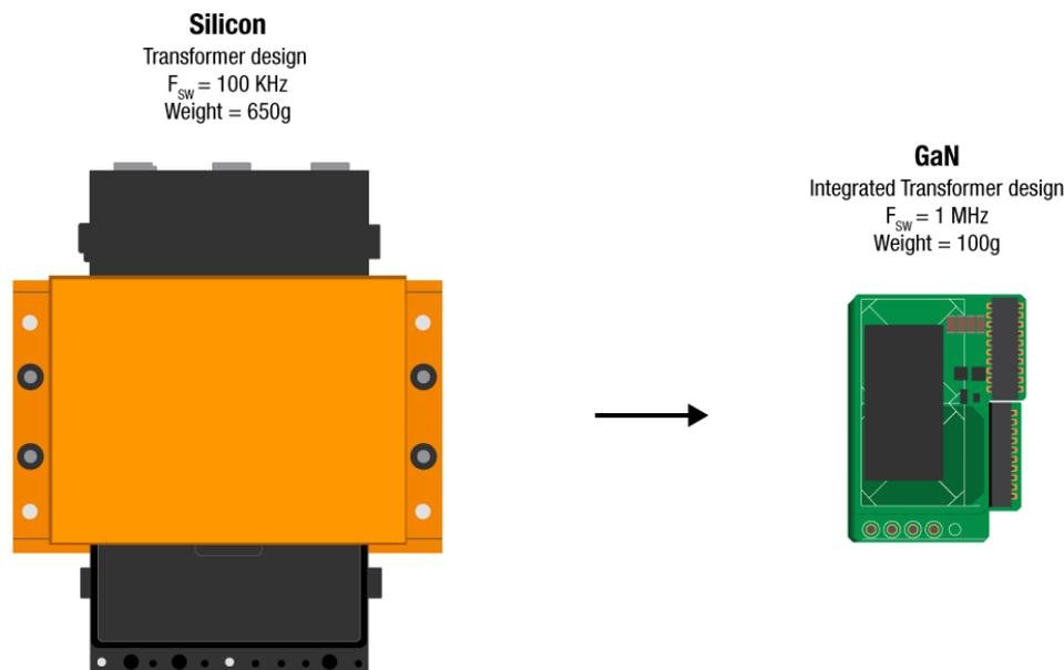
Figure 1. Comparing the power density of the magnetics of silicon designs vs. GaN designs
