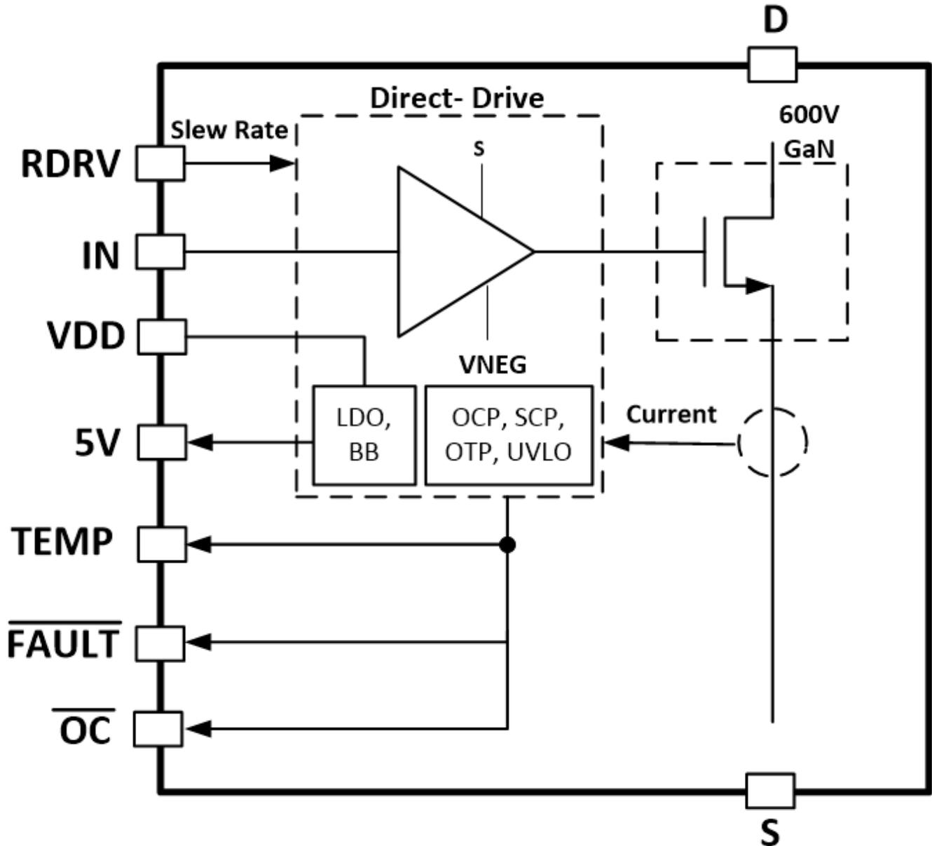
**Figure 2. The integration of a 600-V GaN FET with a gate driver and short-circuit protection**
