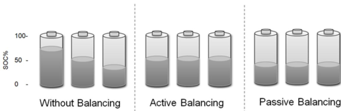
Figure 1. Battery state of charge in various balancing modes
