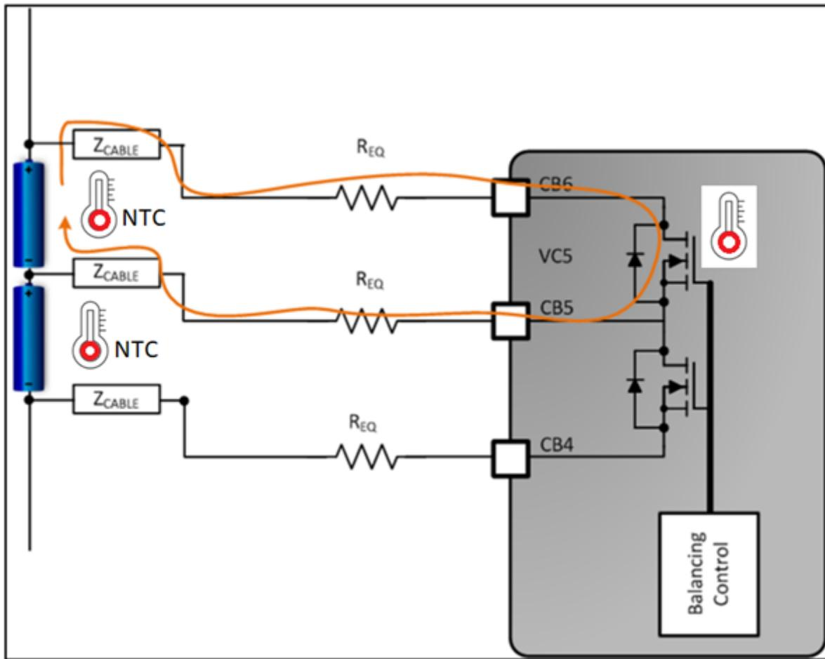
**Figure 2. BQ79616-Q1 temperature monitoring locations on the PCB**
