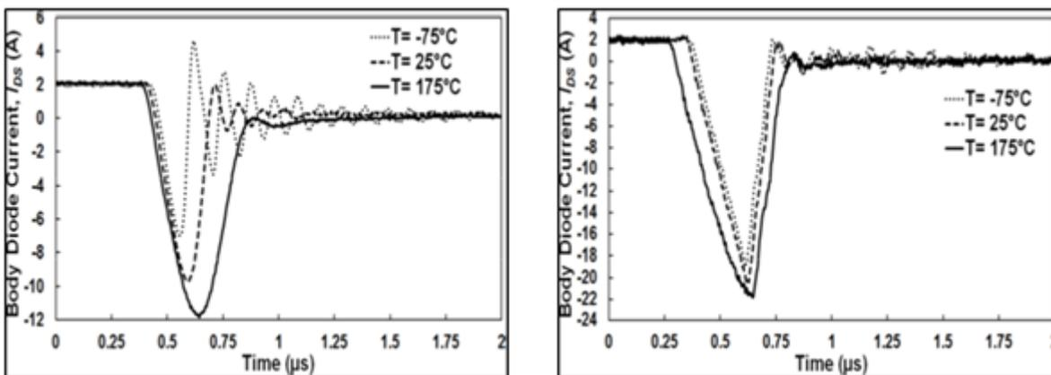
Figure 8. Reverse-recovery current vs. temperature for two FETs
