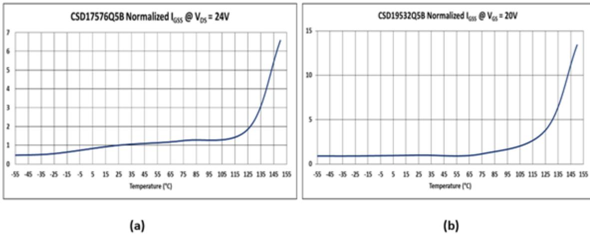
**Figure 5. Normalized  $I_{GSS}$  vs. temperature: CSD17576Q5B (a); CSD19532Q5B (b)**
