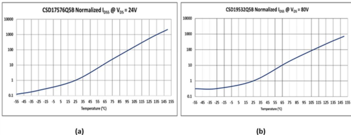
**Figure 4. Normalized  $I_{DSS}$  vs. temperature: CSD17576Q5B (a); CSD19532Q5B (b)**
