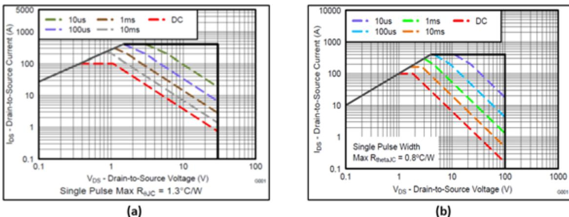
Figure 9. Maximum safe operating area at  $T_A = 25^\circ\text{C}$ : CSD17576Q5B (a); and CSD19532Q5B (b)
