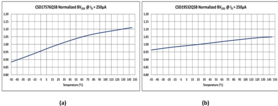
**Figure 3. Normalized  $BV_{DSS}$  vs. temperature: CSD17576Q5B (a); CSD19532Q5B (b)**
