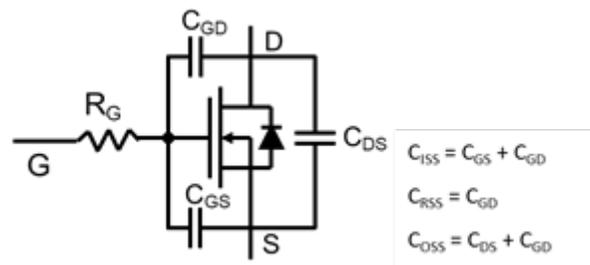
**Figure 7. MOSFET model with parasitic elements**
