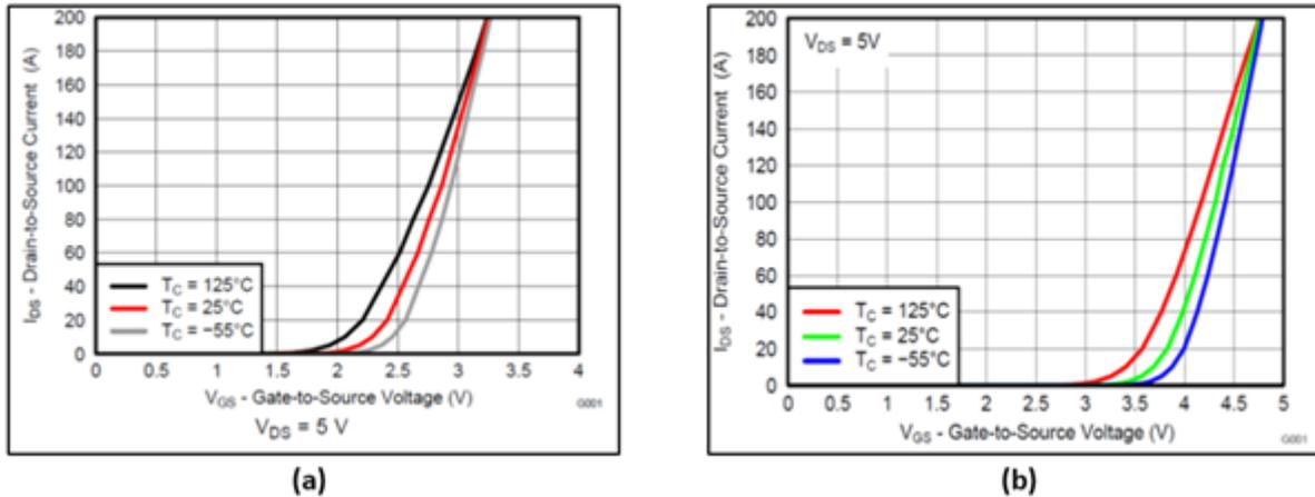
**Figure 6. Transfer characteristics: CSD17576Q5B (a); CSD19532Q5B (b)**
