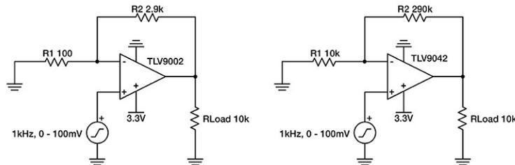
**Figure 4. A typical design vs. a power-conscious design**
