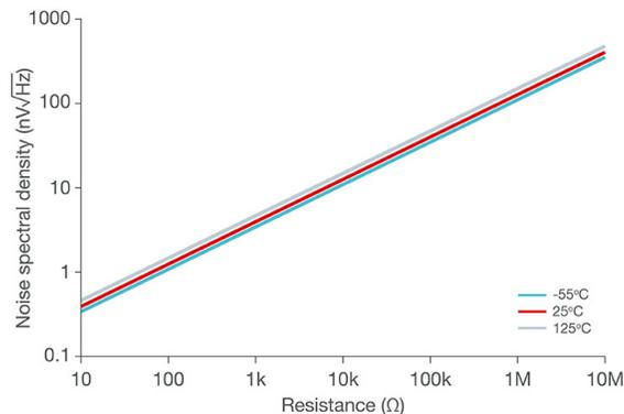
**Figure 3. Resistor thermal noise**
