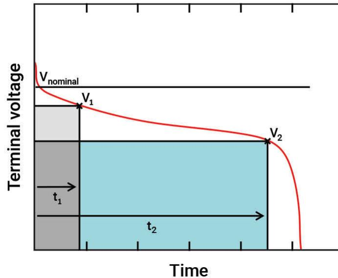
Figure 1. Typical Discharge Curve of a Single-cell Battery
