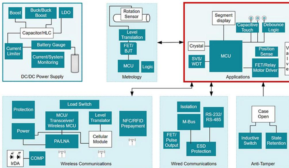
**Figure 3. Reference Design for a Rotary Water Meter**
