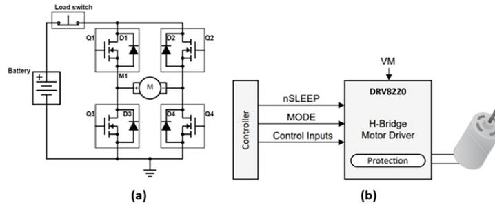
**Figure 2. A Simplified Implementation of an H-bridge with Low-power Sleep Function Using an External Cut-off Switch (a); TI's DRV8210 with Automatic Sleep Mode (b)**
