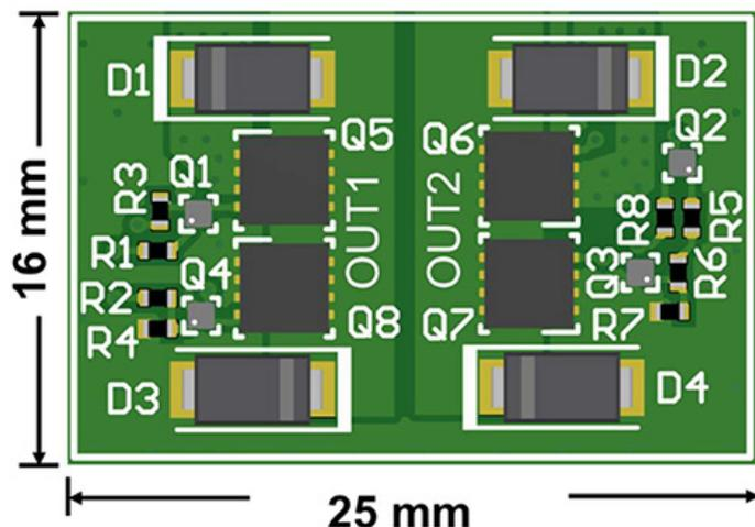
**Figure 4. Discrete Implementation of an H-bridge and the Basic Surrounding Circuit; the PCB Area Is 16 Mm by 25 Mm, or 400 Mm<sup>2</sup>**
