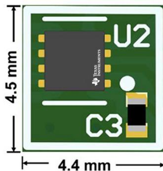
**Figure 5. The DRV8220DSG Integrated Motor-driver Layout; the PCB Area Is 4.5 Mm by 4.4 Mm, or 19.8 Mm<sup>2</sup>**
