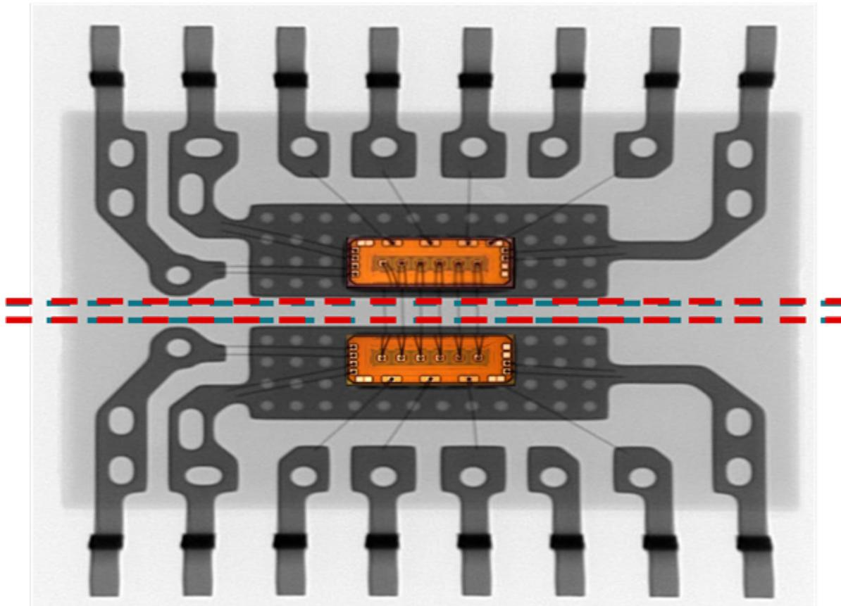
**Figure 1. The Internal Architecture of a Digital Isolator Includes a Split Leadframe and Requires Separate Primary and Secondary Supplies**
