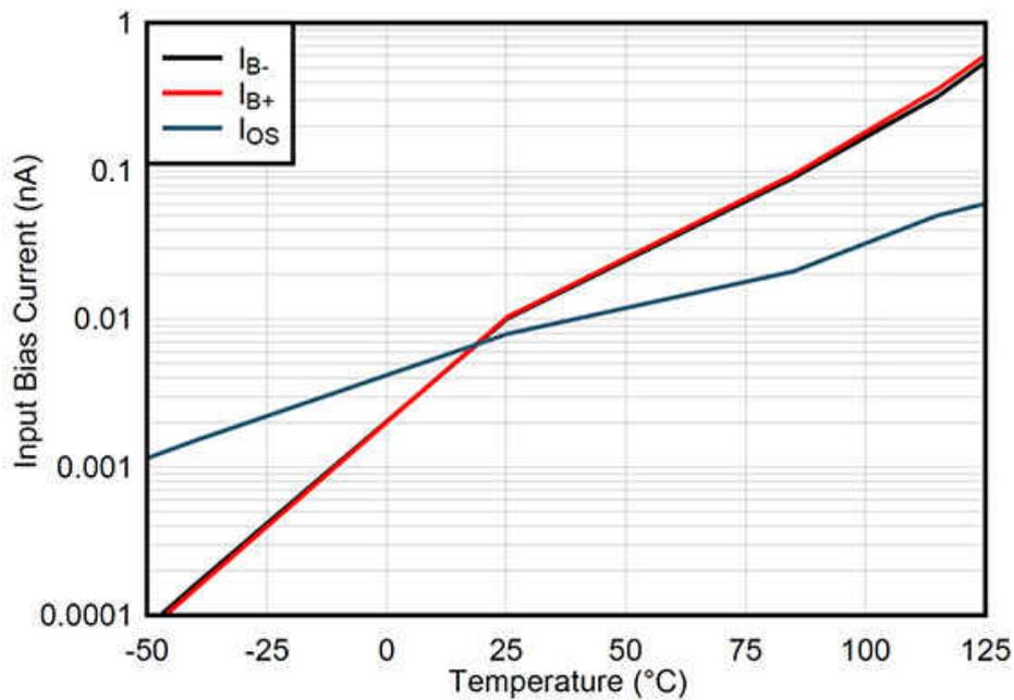
Figure 2. The OPA2205'S Input Bias Current over Temperature
