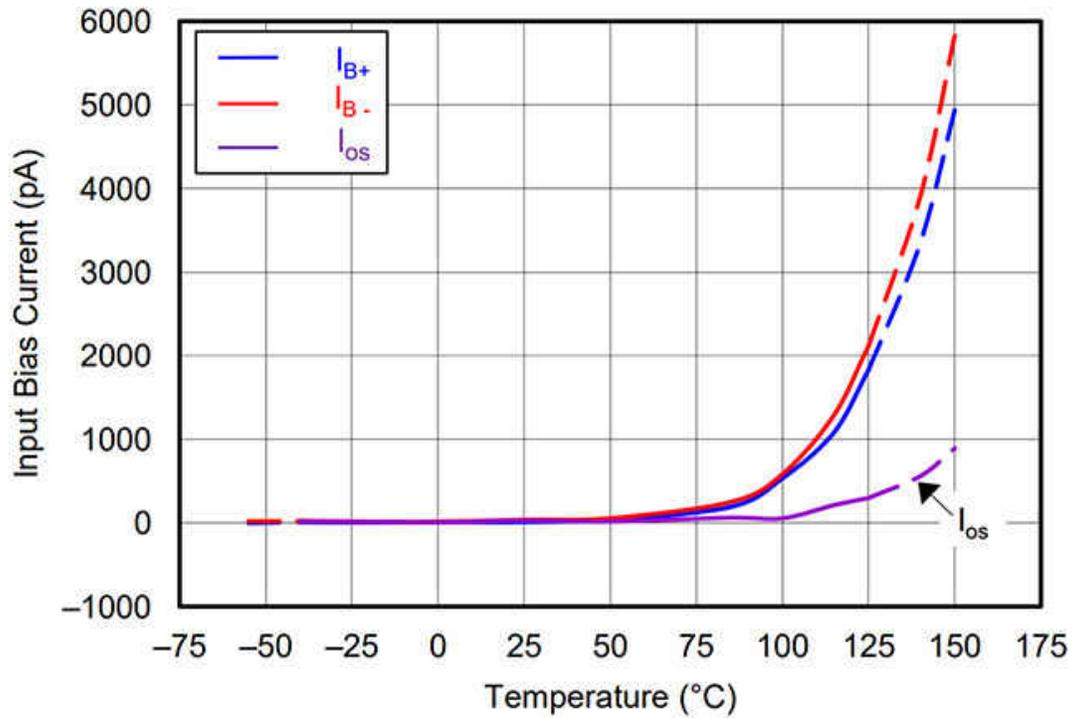
Figure 1. An OPAx192'S Input Bias Current over Temperature
