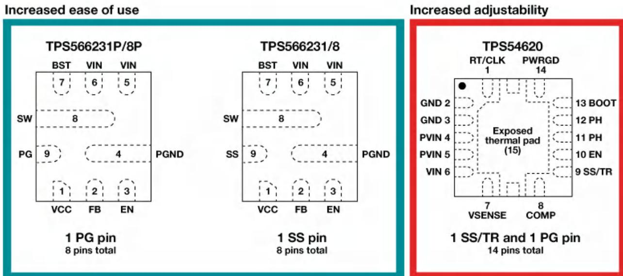
**Figure 2. TPS566231/1P/8/8P Pinout vs TPS54620 Pinout**
