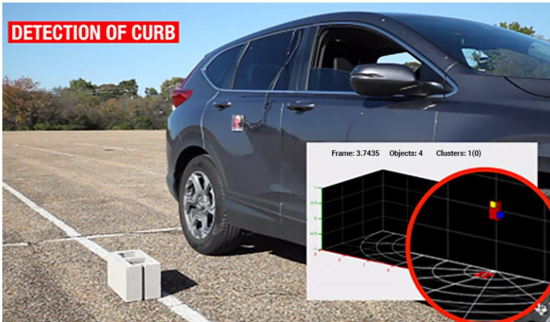
**Figure 2. Detection of a Low-height Cinder Block Acting as a Curb Using TI's AWR1843AOP EVM**
