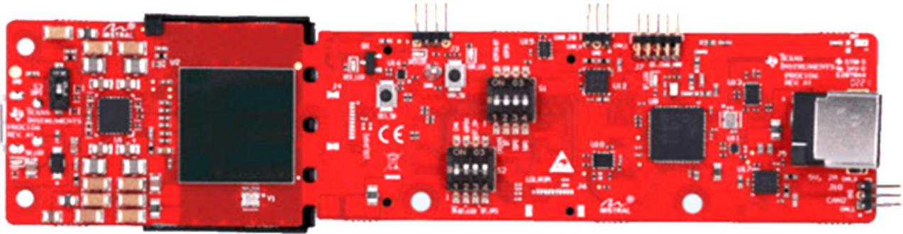
**Figure 4. TI's AWR1843AOP mmWave Radar Sensor**
