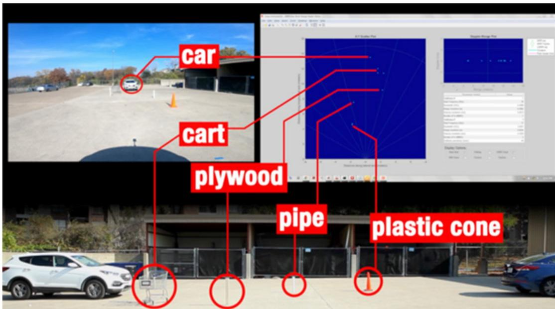
**Figure 3. Detecting Multiple Static Objects of Various Types, Sizes and Materials**
