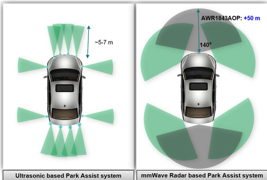
**Figure 1. Comparison of Range and Field of View for Ultrasonic vs. mmWave Radar Systems**
