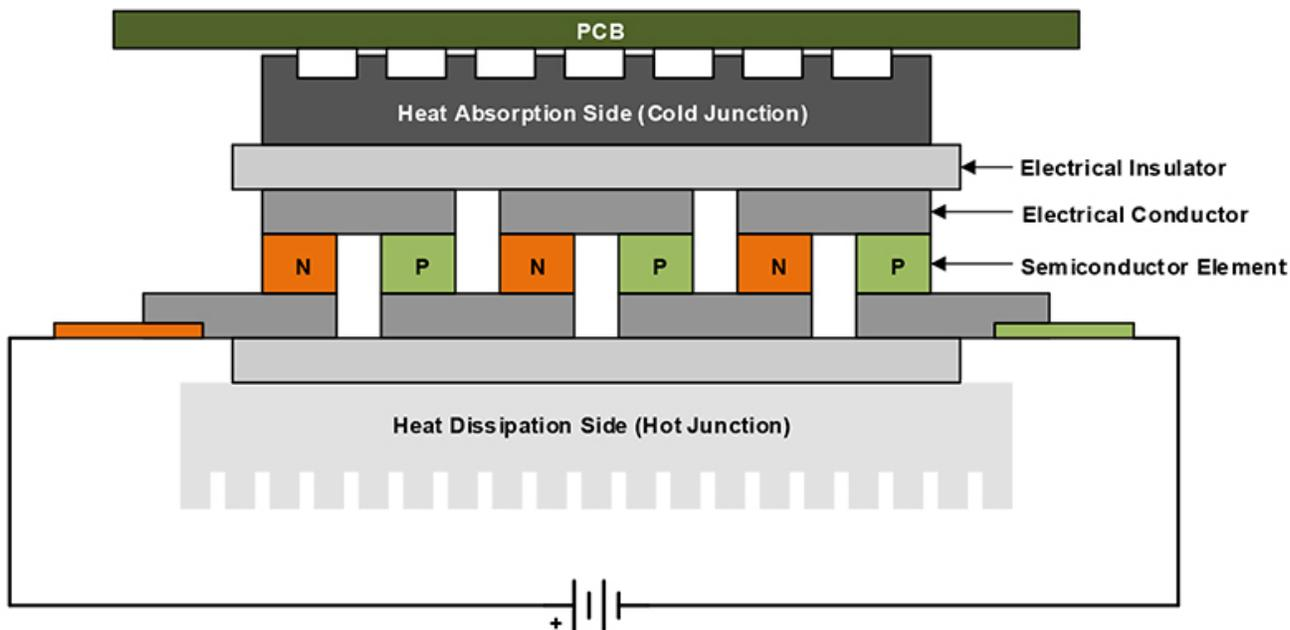
**Figure 1. Semiconductor-based Peltier Element**
