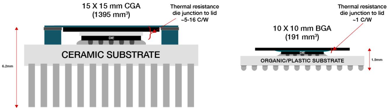
**Figure 1. Comparing Hermetic-ceramic Packaging to Plastic Packaging**
