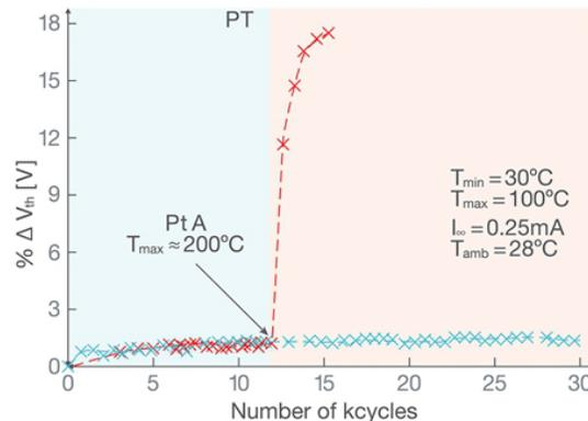
Source: "Analysis of  $V_{th}$  Variations in IGBT under Thermal Stress for Improved Condition Monitoring in Automotive Power Conversion Systems"
