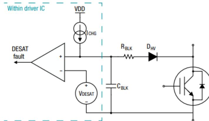
Figure 1. Typical Desat Circuit Implementation
