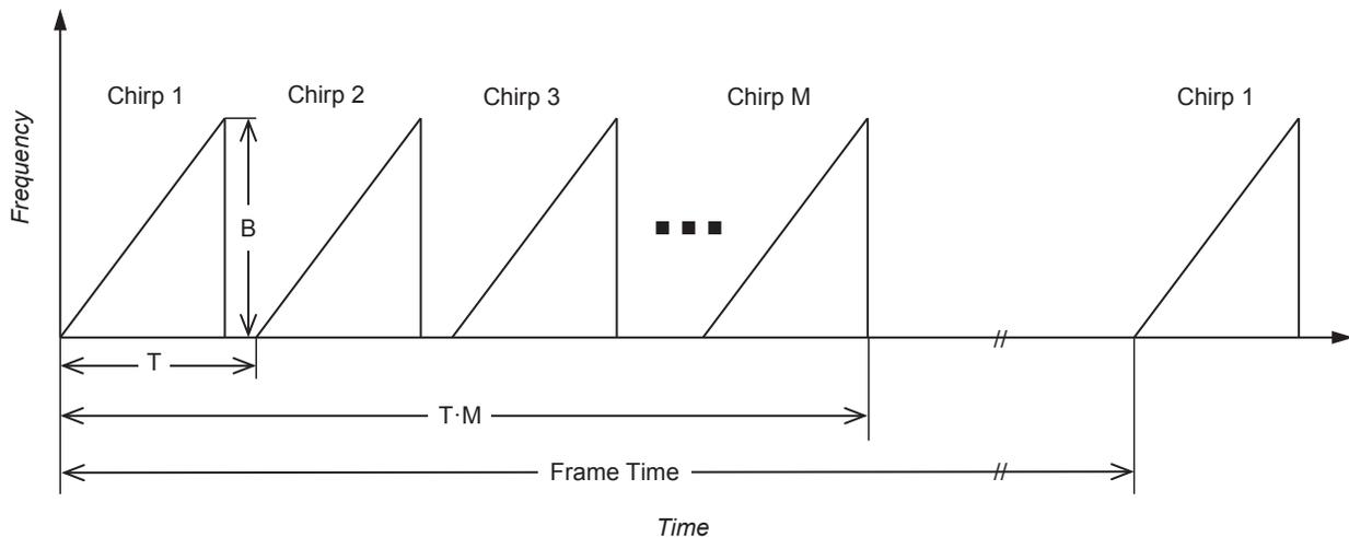
**Figure 4.** Frequency vs. time graph depicting a fast FMCW frame where  $B$  is the chirp bandwidth,  $T$  is the chirp repetition time (which could be a few tens of microseconds) and  $T \cdot M$  is the total active chirping time in one frame. The frame time includes an idle time that may be a few tens of milliseconds.
