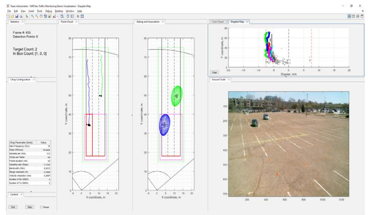
**Figure 7.** Two moving vehicles as detected by the example medium-range MIMO configuration. The graph on the right shows the detection of two vehicles around 40 m and 60 m, separated in angle for lane detection. The color of the points indicate the different Doppler measurements of the vehicles around 6 m per second (22 kph) and 8 m per second (29 kph).
