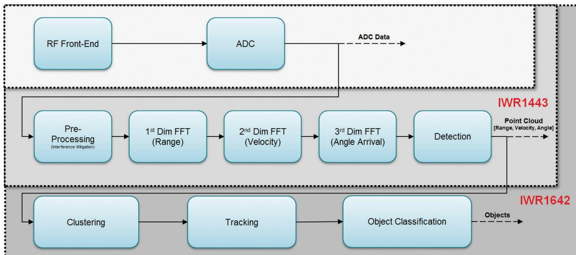
**Figure 2.** mmWave signal processing chain.
