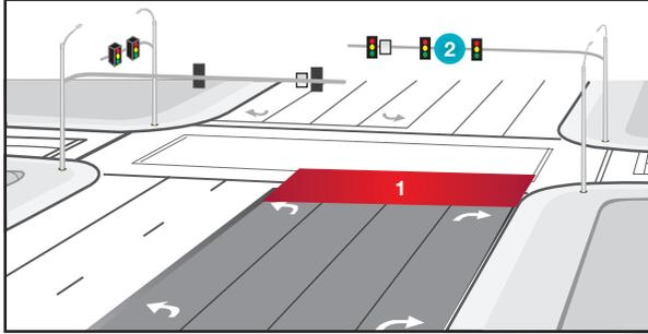
**Figure 1.** Example intersection where traffic sensors can be positioned at the stop bar (1) or on the traffic pole (2). Sensors mounted on the traffic pole are advantageous in that they do not require installation in the road surface.
