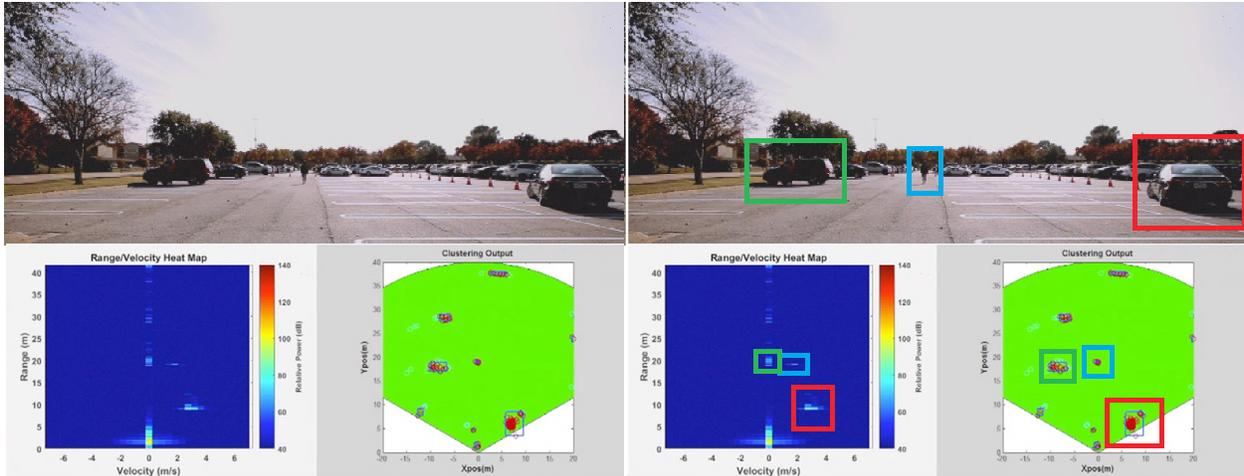
**Figure 3.** Range, velocity and angle information from mmWave sensors in an example parking lot scene. The graph with the blue background is a range/velocity heat map, where moving and nonmoving objects and their velocities are identifiable; the graph with the green background is a range/angle visualization. Colored boxes highlight the moving and nonmoving vehicles and pedestrians in the scene.
