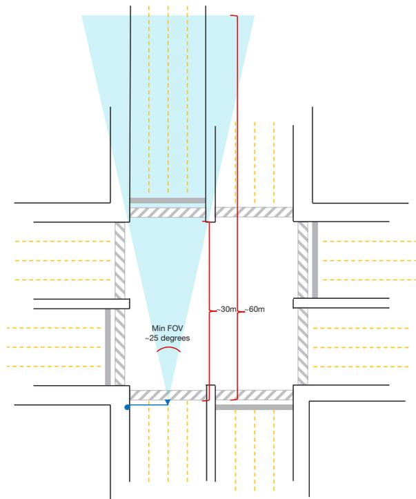
**Figure 5.** Example intersection with overhead radar sensor mount and azimuth field of view of 25 degrees covering a four-lane stop bar at a distance of approximately 30 m and an approach of approximately 60 m.
