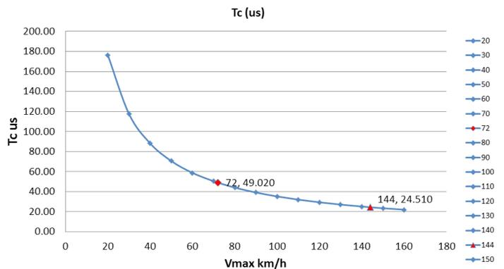
Figure 4. Maximum measurable velocity vs. chirp duration/period total
