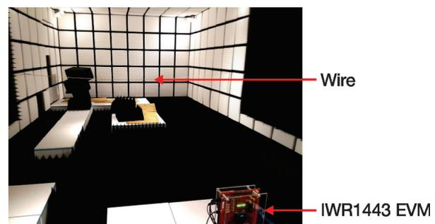
**Figure 7.** Anechoic chamber test setup for wire-line testing
