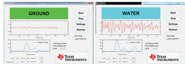
**Figure 6.** Using mmWave to detect ground or water surfaces
