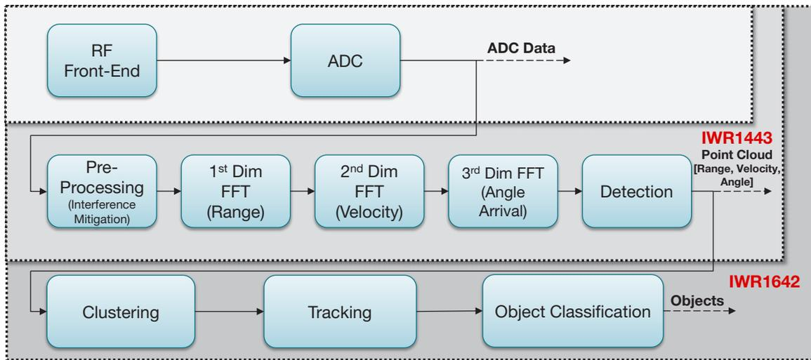
Figure 1. mmWave signal processing
