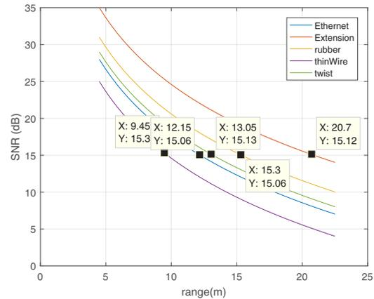
**Figure 9.** Detection range extrapolation by wire type
