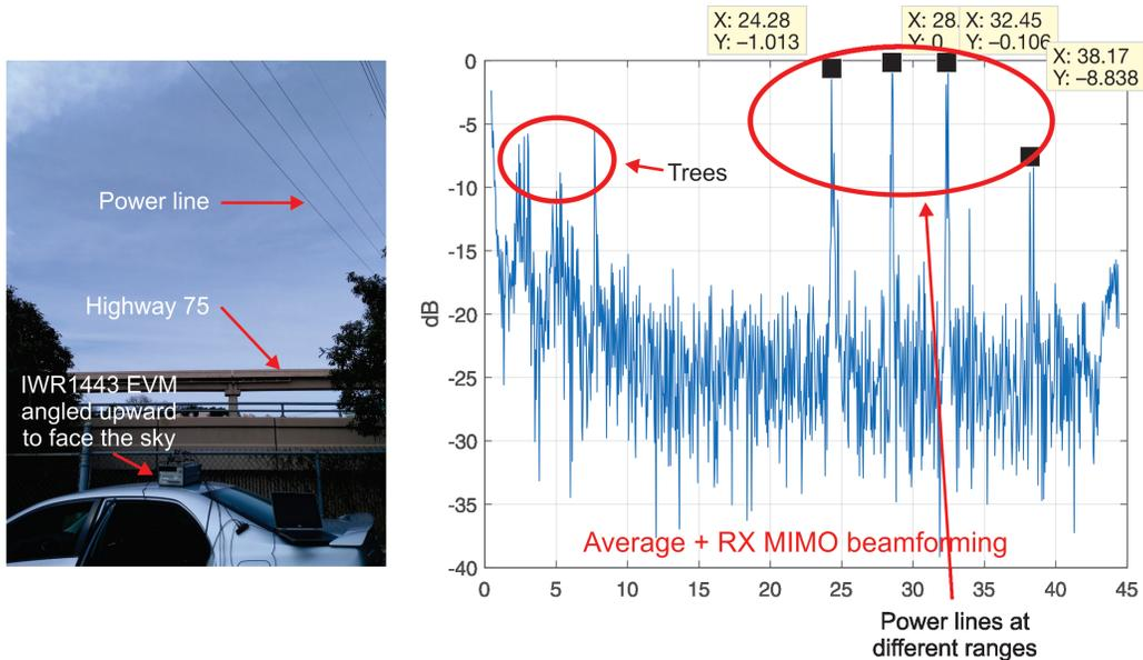
Figure 10. Outdoor power-line detection with the IWR1443 EVM
