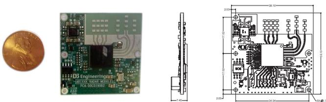
Figure 3. Typical mmWave module design
