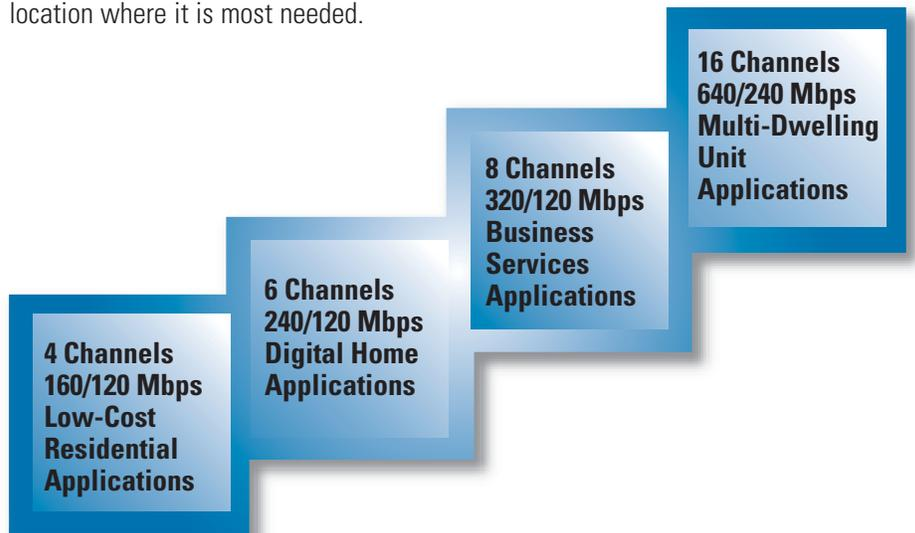
**Figure 1:** DOCSIS 3.0 is extremely flexible and scalable. With its channel bonding technology, multiple channels can be bonded together to achieve the line speed and bandwidth needed by a particular segment of the local marketplace.
