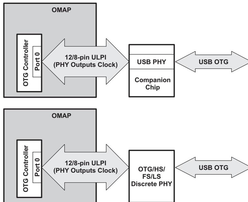
Figure 12. Typical Uses for USB Port 0
