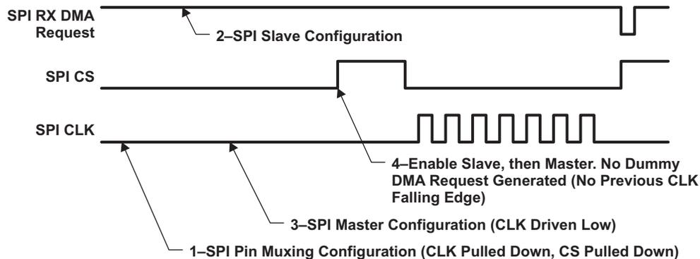
**Figure 6. Dummy DMA RX Generation (No Clock Edge)**
