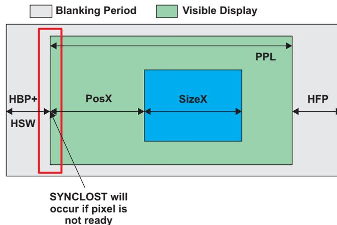
Figure 2. Synclost Interrupt
