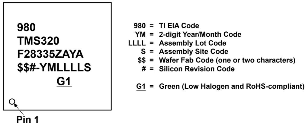
Figure 2-2. Example of Device Markings (ZAY)
