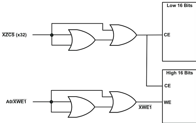
**Figure 4-3. Example Delay Line Circuit**
