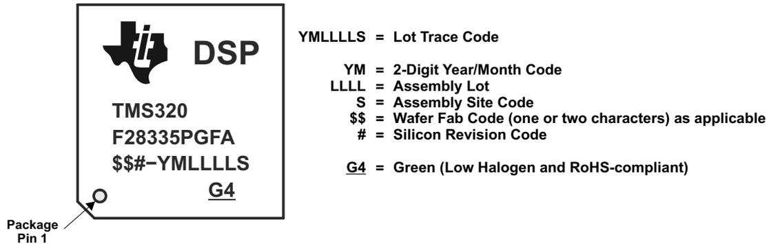
Figure 2-1. Example of Device Markings (PGF)
