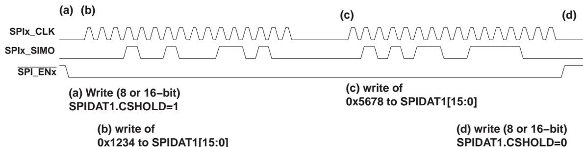
**Figure 6. Workaround Assuming Halfword Writes to SPIDAT1**
