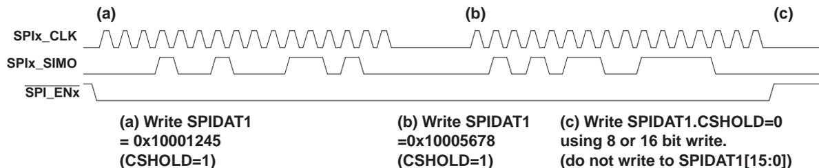
**Figure 5. Workaround Assuming 32-Bit Writes to SPIDAT1 Followed by a Write Only to CSHOLD**
