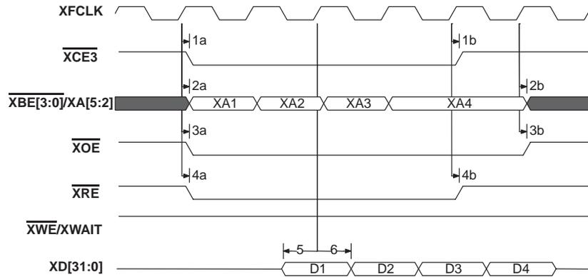
**Figure 7. FIFO Read Timing, Glueless Read Mode**
