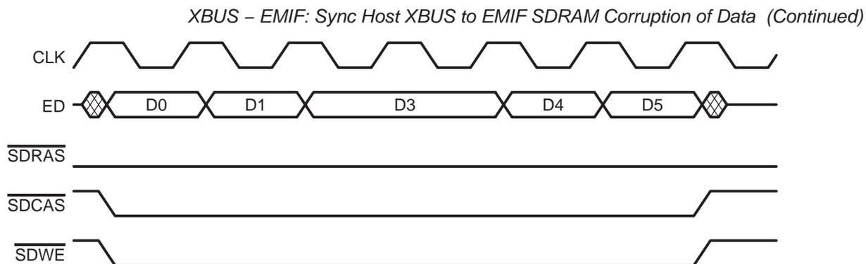
**Figure 3. Failing Transfer as Seen at Destination**
