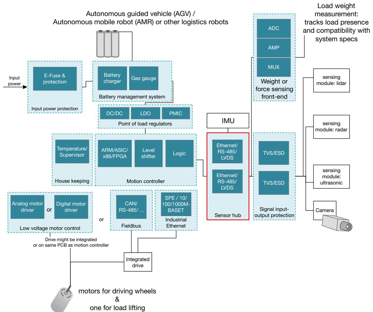
**Figure 2:** High level block diagram for an autonomous guided vehicle or robot.
