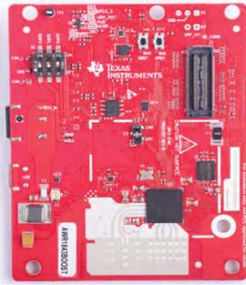
**Figure 6.** TI's AWR1843BOOST 77-GHz Automotive mmWave Evaluation Module
