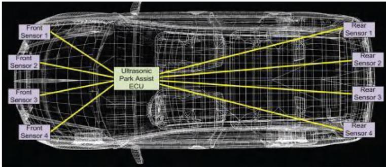
**Figure 2.** Placement of Ultrasonic Sensors around an Automobile for Varying Degrees of Object Detection Coverage
