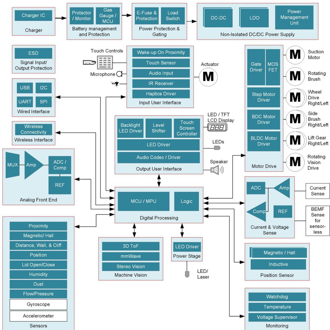
Figure 1: TI vacuum robot reference diagram.
