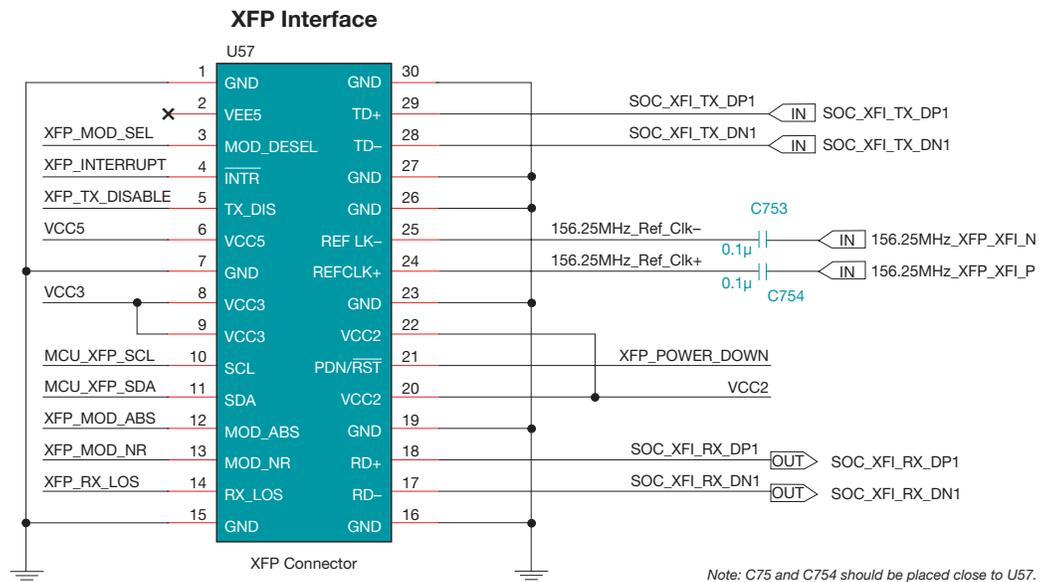
**Figure 5: Typical electrical interface for XFI-to-XFP connector**
