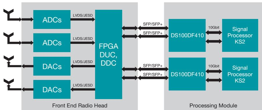
**Figure 4: Proposed radar system with SFP+ interface with the supplemental hardware DS100DF410 retimer for converting XFI to SFI interface**
