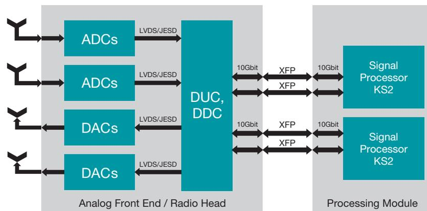
Figure 3: Proposed radar system with XFP interface
