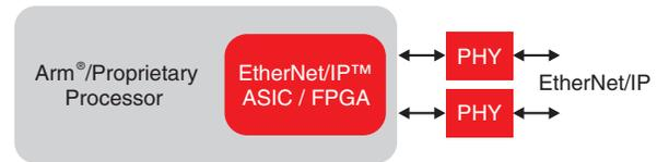
**Figure 8.** Integrated EtherNet/IP with processor.
