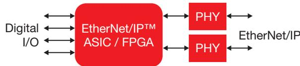
**Figure 6.** Basic digital I/O EtherNet/IP node.
