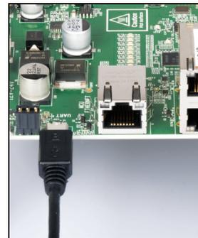
**5** Optional: If you plan to use Code Composer Studio (CCS) IDE to control the IDK, you must use another USB cable connected to the USB connector labeled “XDS110\_USB” on the board. Refer to [http://software-dl.ti.com/processor-sdk-rtos/esd/docs/latest/rtos/How\\_to\\_Guides.html#host](http://software-dl.ti.com/processor-sdk-rtos/esd/docs/latest/rtos/How_to_Guides.html#host) for details about CCS setup.
