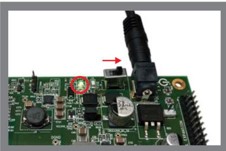
**4** Connect 12V power cable to the DC jack (J3). Slide the power switch SW1 to the "ON" position marked on the silkscreen. LED LD9 will light up.
