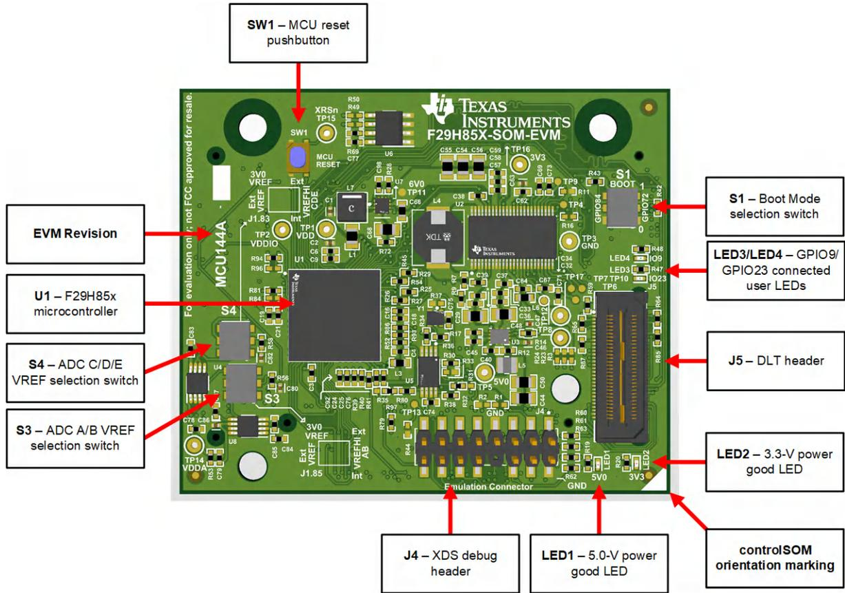
Figure 1-2. Key Components on the controlSOM - Front
