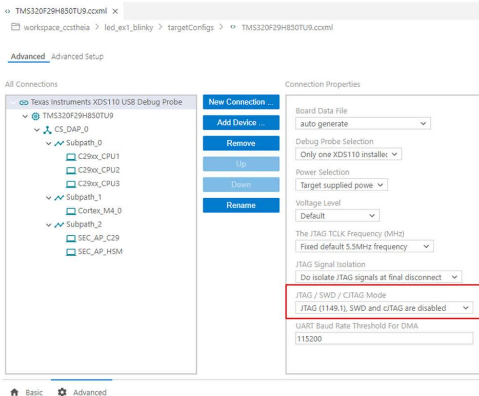
**Figure 2-14. Target Configuration Advanced Options**
