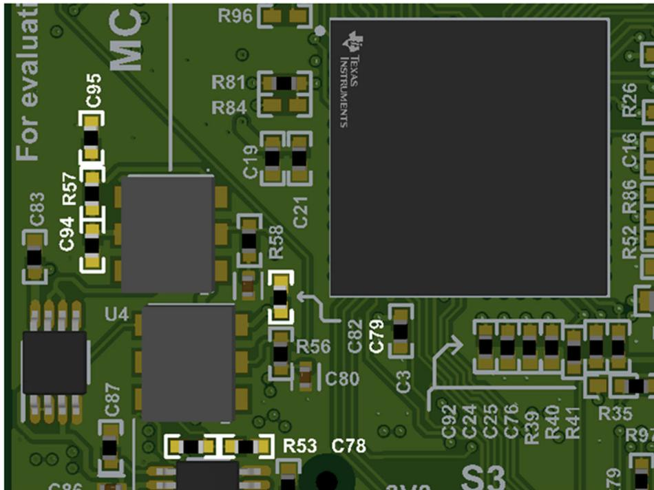
**Figure 5-1. Component Location For ADC VREF Modification**
