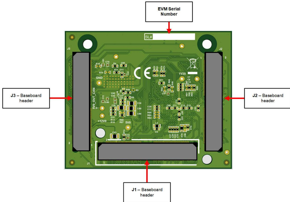
Figure 1-3. Key Components on the controlSOM - Back
