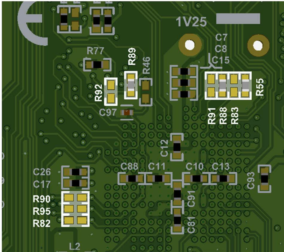
Figure 2-13. FSI DLT Selection Resistor Locations (Bottom)
