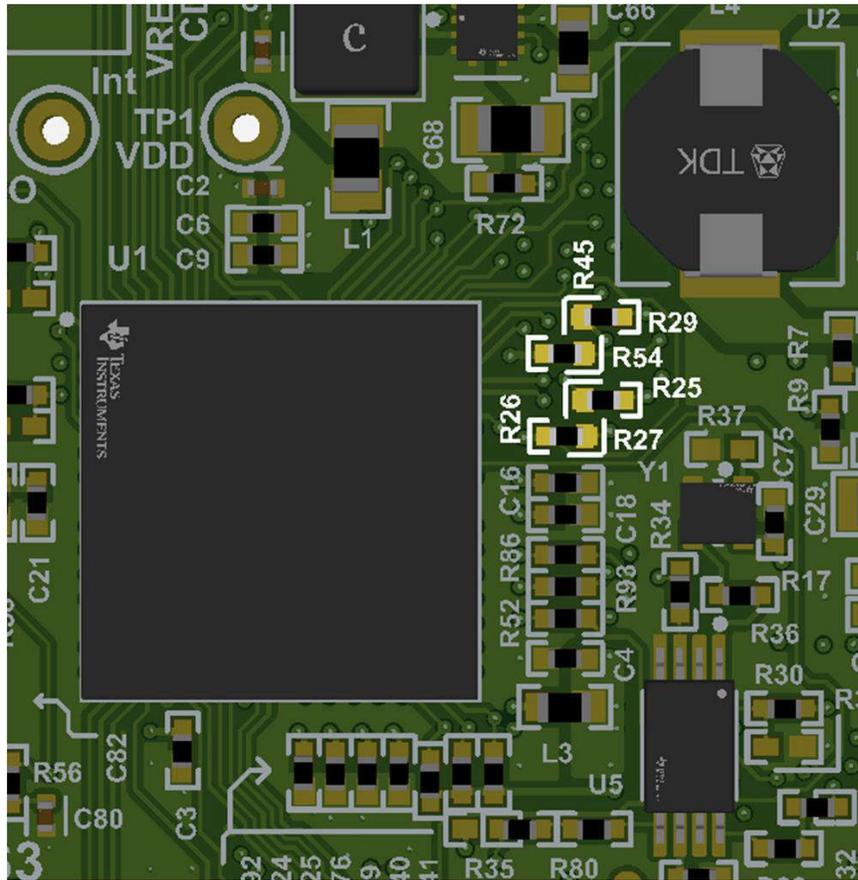
Figure 2-10. MCAN-A Boot Selection Resistor Locations
