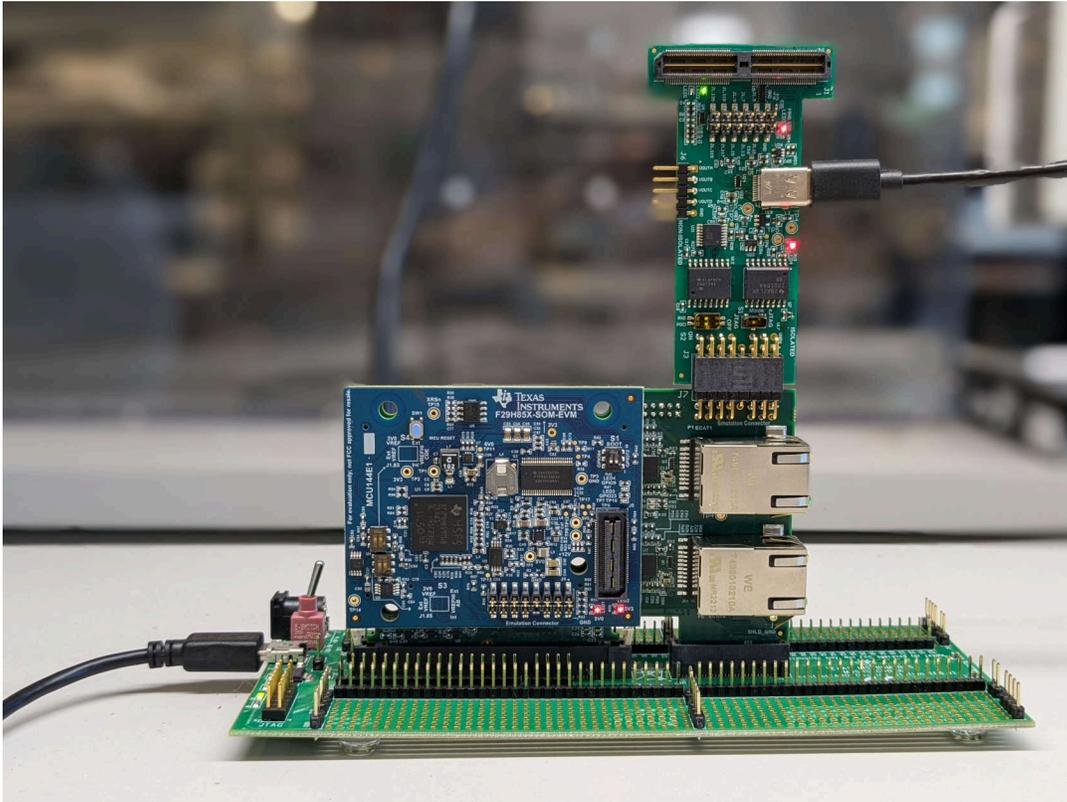
**Figure 2-2. C2000 controlCARD Compatibility Configuration Using HSEC180ADAPEVM**
