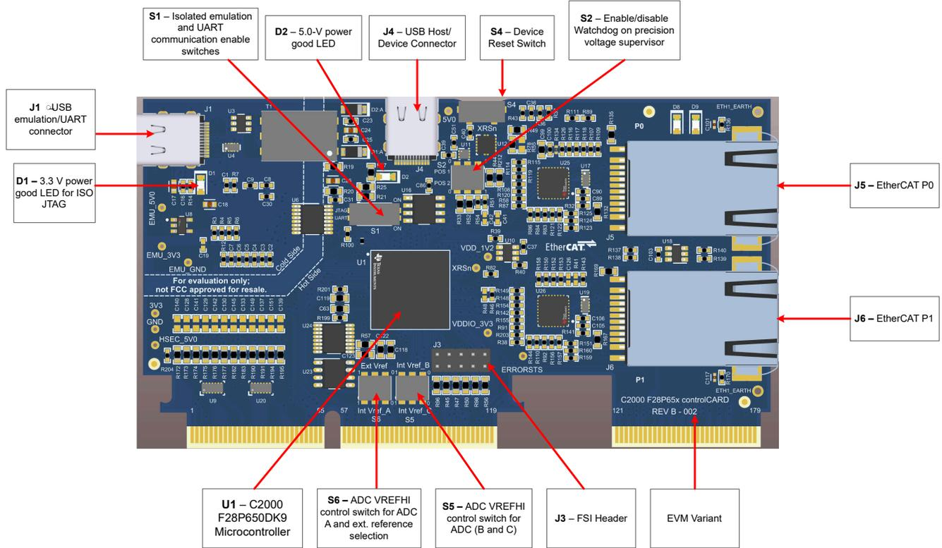
Figure 6-1. Key Components on the controlCARD - Front
