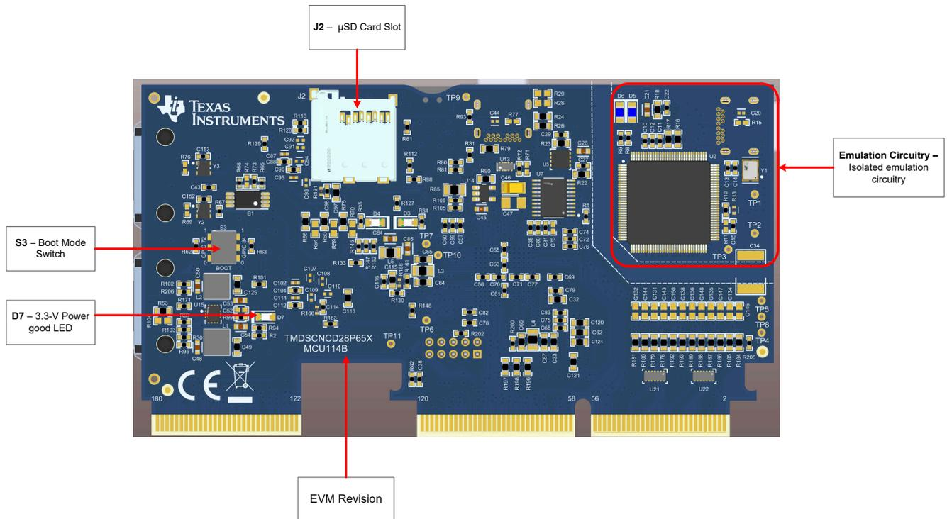
Figure 6-2. Key Components on the controlCARD - Back
