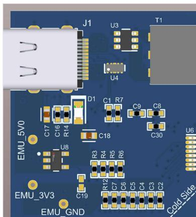
**Figure 5-1. XDS110 Emulation Circuitry and Isolation Circuitry**
