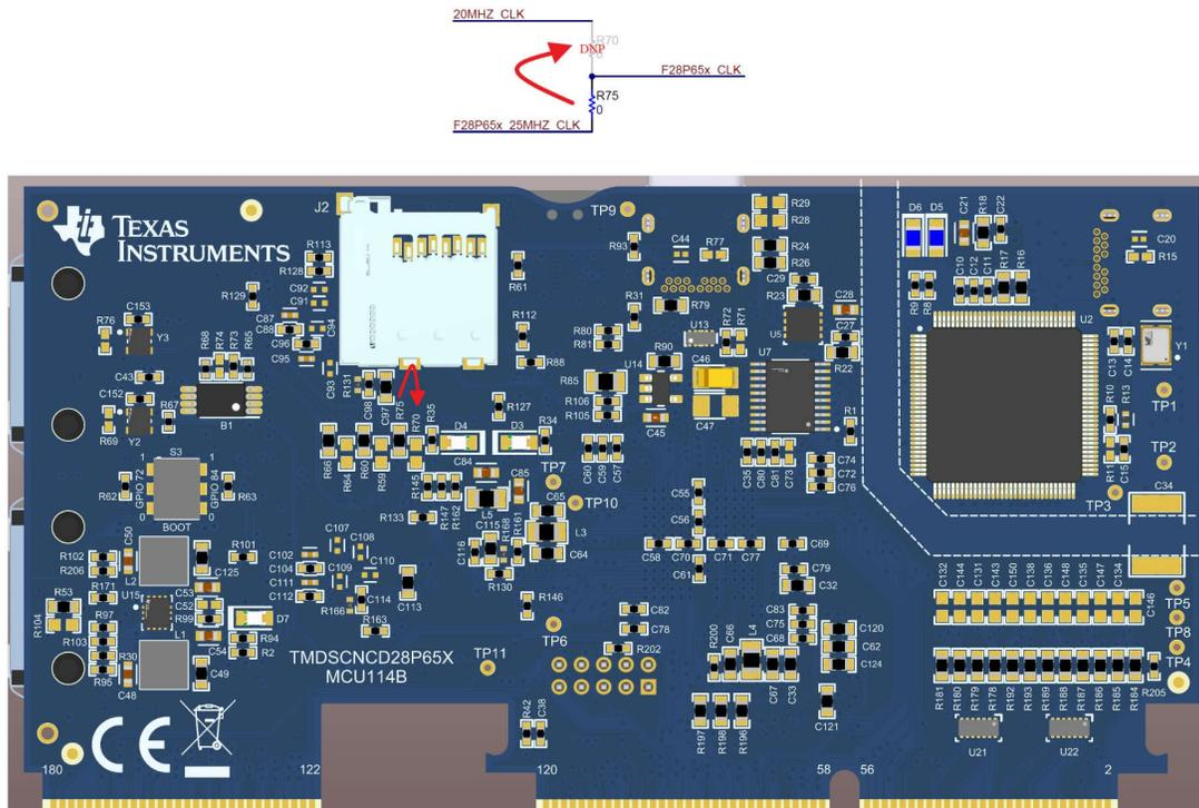
Figure 4-1. Changing the Clock Source From 25MHz to 20MHz
