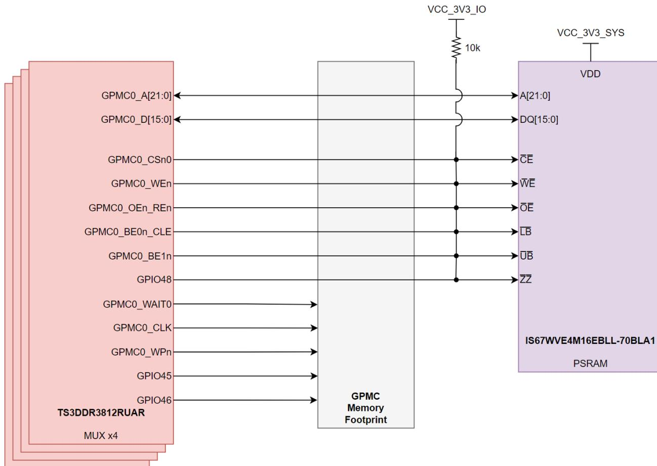
Figure 2-12. GPMC-PSRAM Interface
