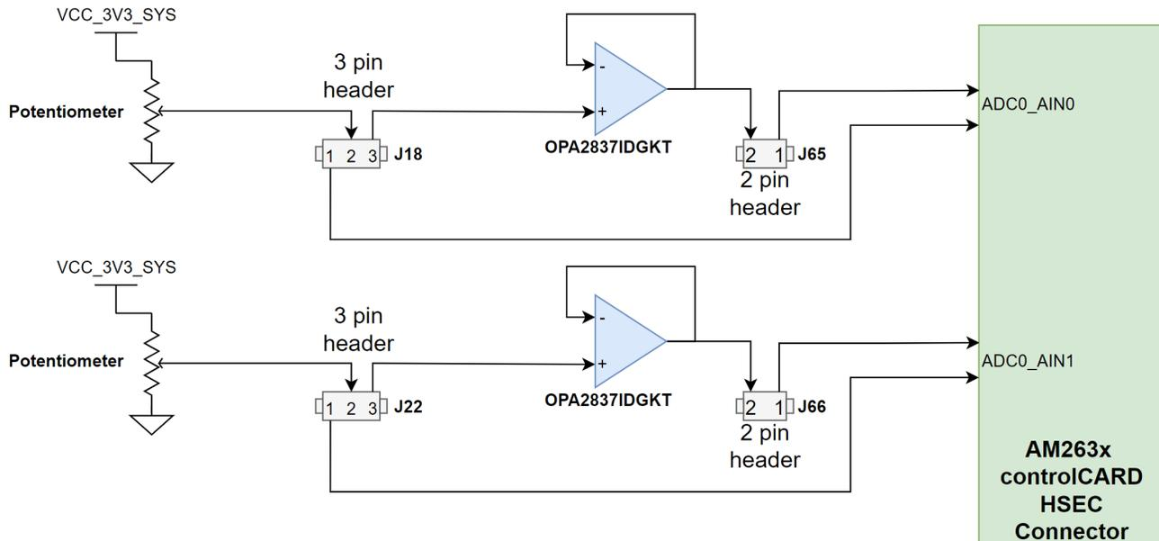
**Figure 2-7. Variable ADC Inputs with Signal Conditioning**
