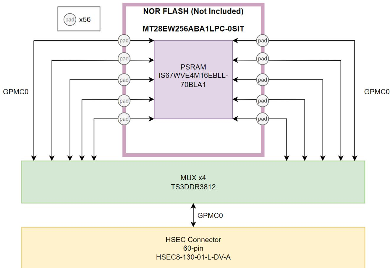
Figure 2-11. AM263x controlCARD Docking Station GPMC Peripheral Functional Block Diagram
