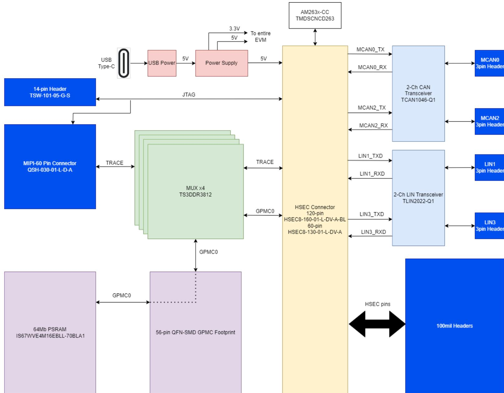
Figure 2-6. AM263x controlCARD Docking Station Functional Block Diagram
