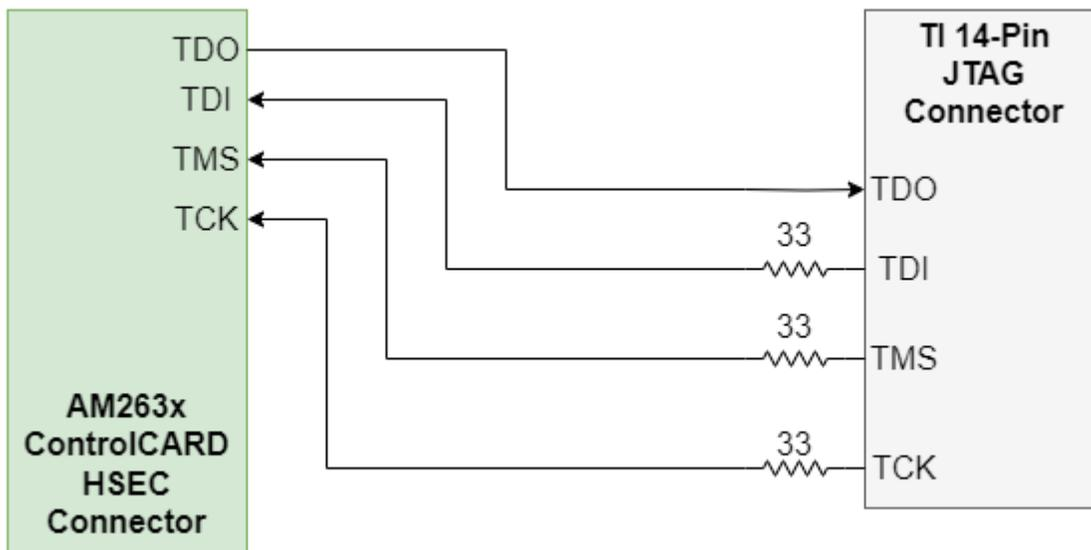
Figure 2-15. TI 14-Pin Header
