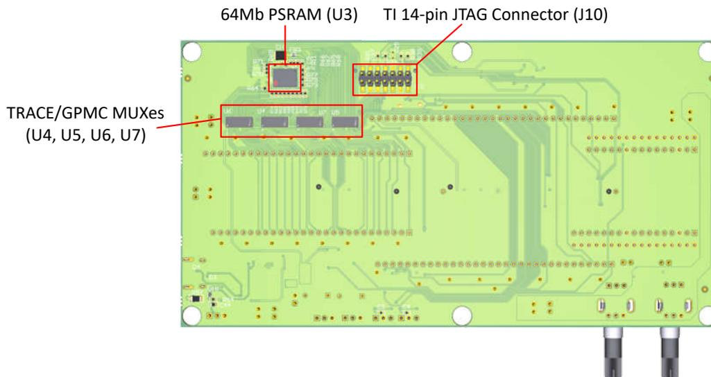
Figure 2-2. AM263x controlCARD Docking Station Bottom Component Identification
