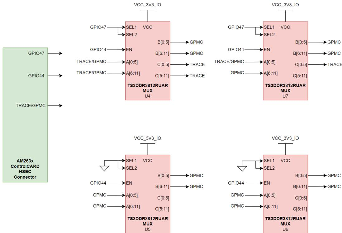
Figure 2-10. TRACE/GPMC Signal Muxing
