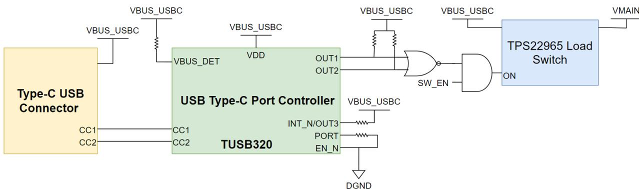
**Figure 2-4. Type-C CC Configuration**
