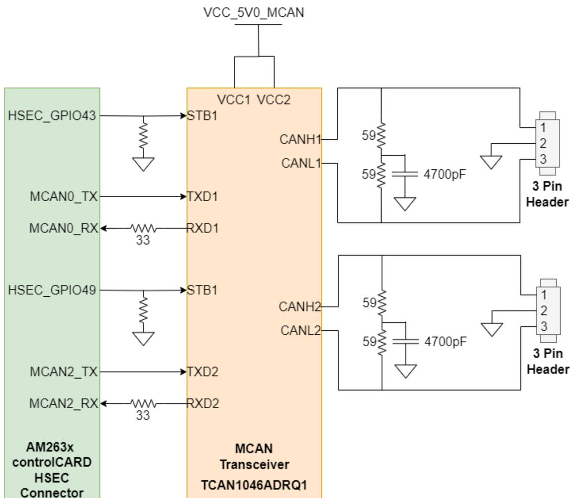
**Figure 2-9. MCAN Transceiver**
