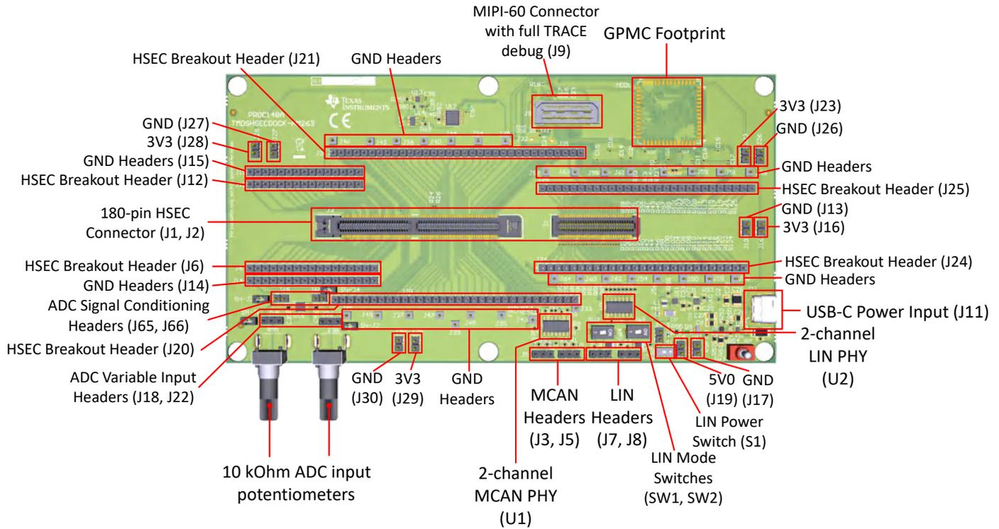
Figure 2-1. AM263x controlCARD Docking Station Top Component Identification
