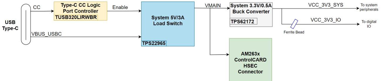
**Figure 2-5. Power Tree Diagram of AM263x controlCARD Docking Station**
