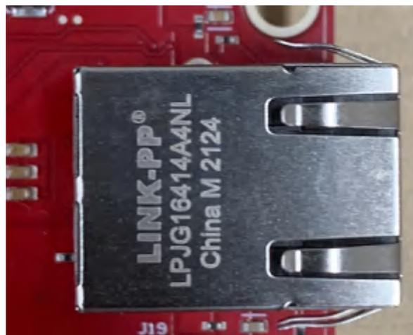
**Figure 2-12. RJ45 Connector**
