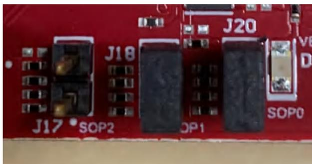
**Figure 2-28. SOP Jumpers**
