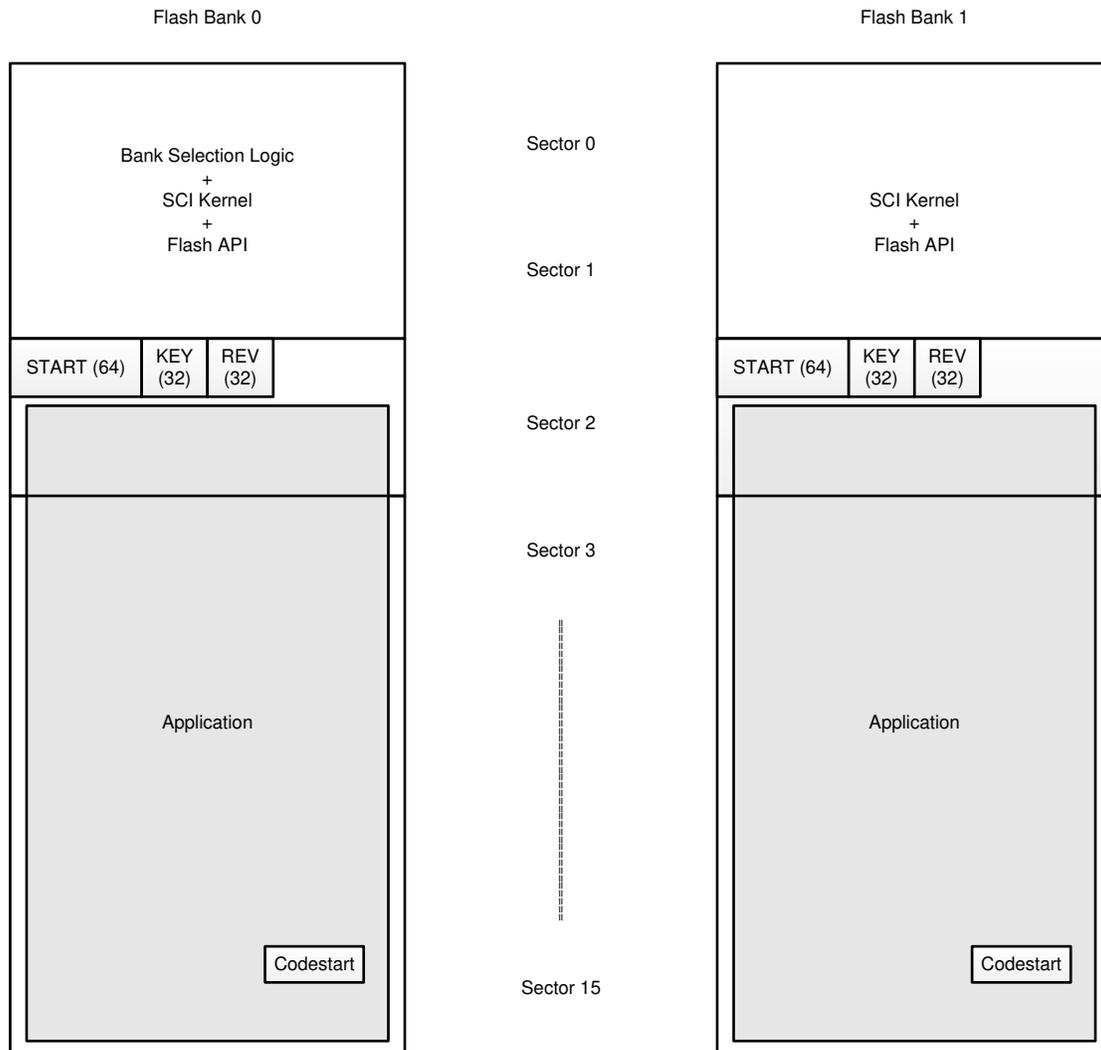
**Figure 3-1. Flash Memory Contents for Bank 0 and Bank 1**
