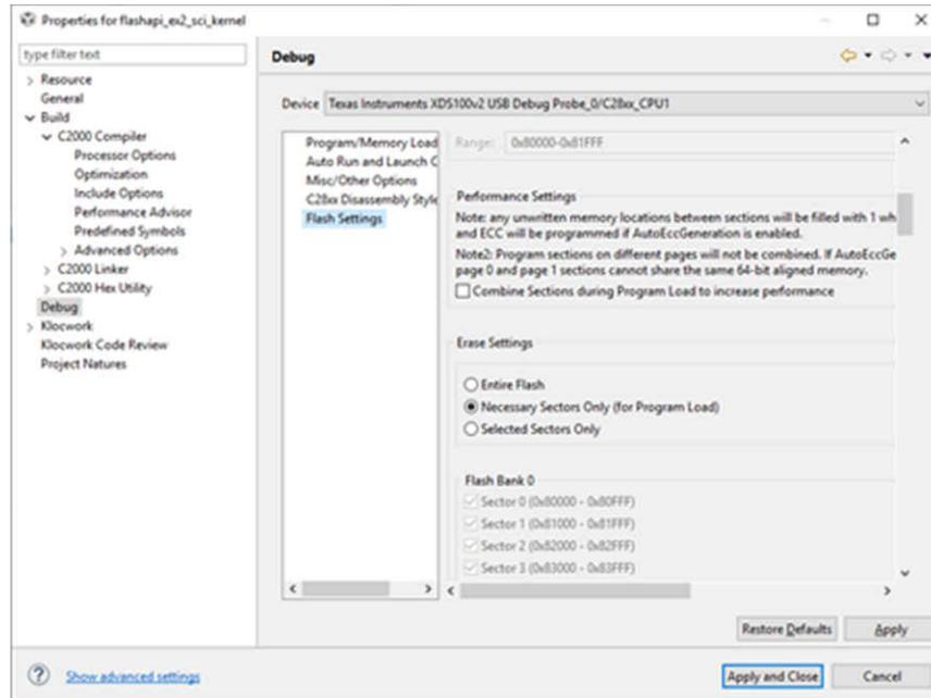
**Figure 6-1. Flash Settings to Only Erase Necessary Sectors**
