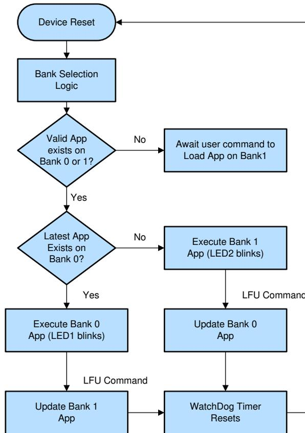
**Figure 6-15. LFU Code Flow Diagram**
