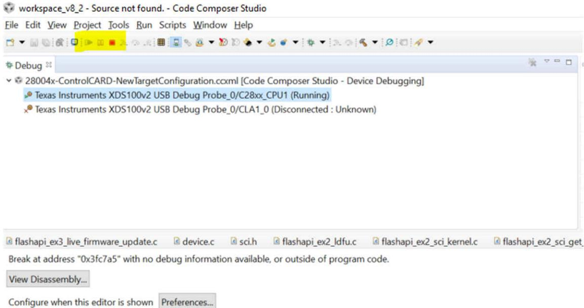
**Figure 6-3. CCS Window view After Programming Bank 0 Flash Kernel**
