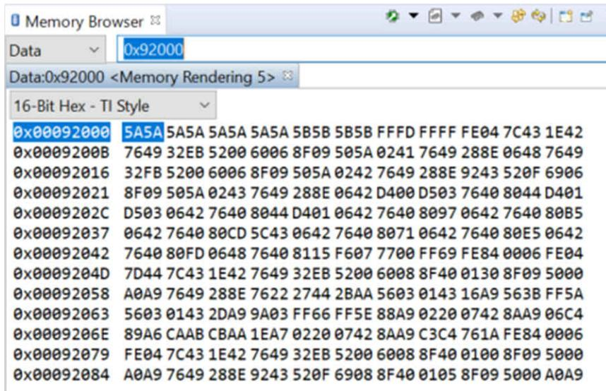
Figure 6-7. CCS Memory Browser View to Verify Successful Programming of Application on Bank 1
