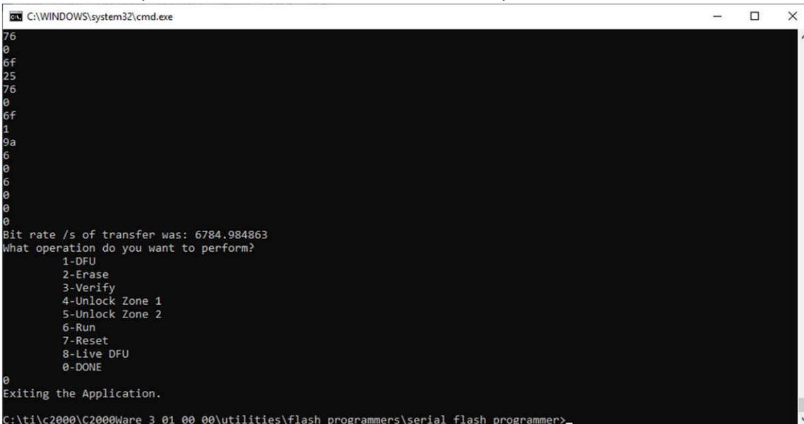
**Figure 6-12. Successful Completion of LFU Command to Program Flash Bank 0**
