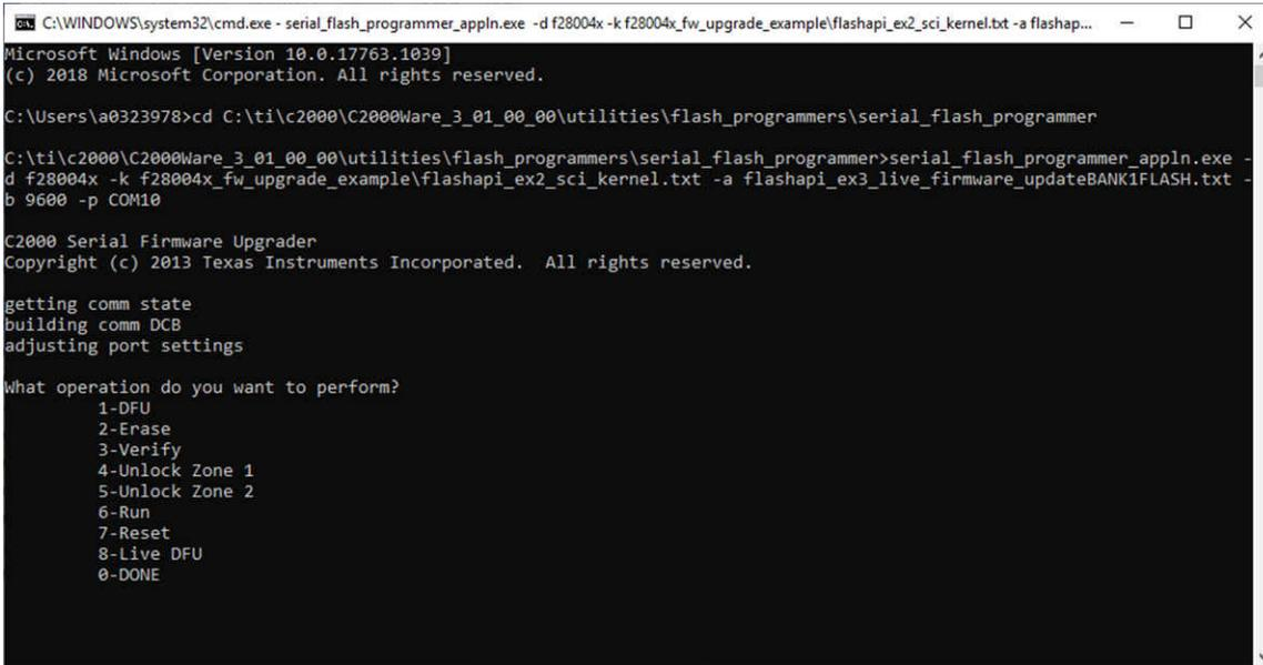
**Figure 6-11. LFU Serial Command Invoked From Windows Command Prompt**
