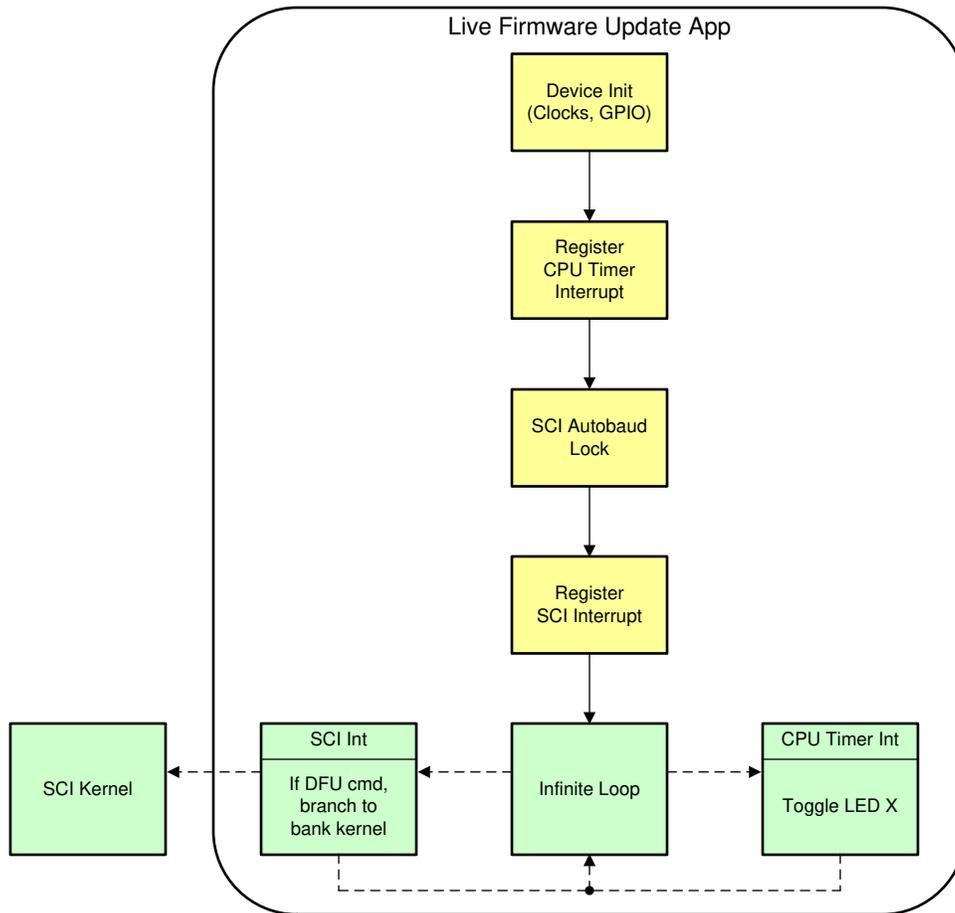
**Figure 5-1. Code Flow After Entering main() of Application**
