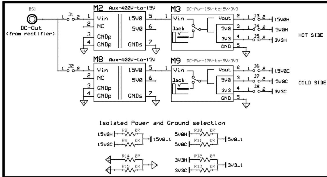
Figure 2-12. Schematic Configuration of Power Supplies
