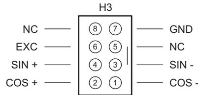
Figure 2-7. Resolver Interface Header
