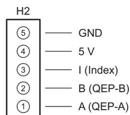
Figure 2-6. QEP Interface Header
