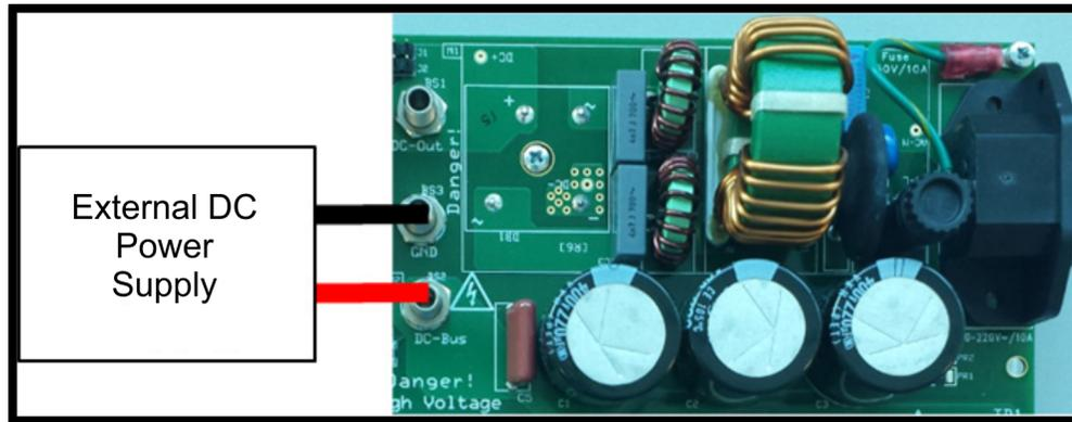
Figure 2-16. Powering Through an External DC Source
