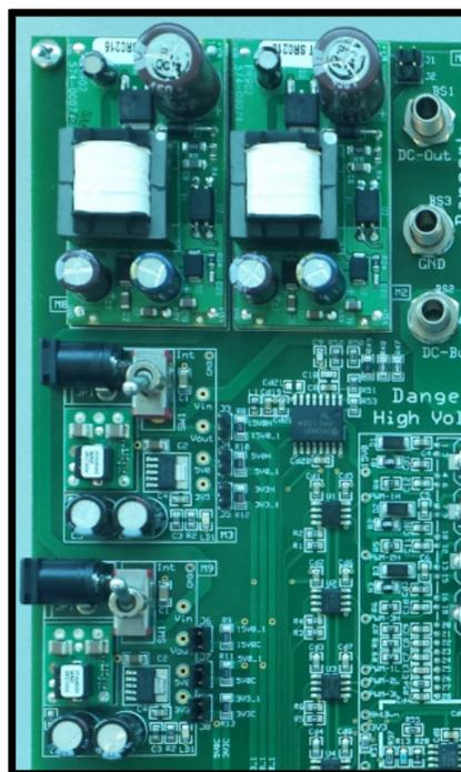
Figure 2-11. Power Supply Block
